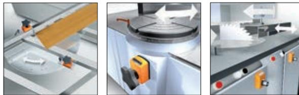
E.g., angle adjustment units on saws, rotary and milling tables
