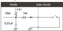
For output circuit: the pull-up resistance must be set not to over 10mA.
