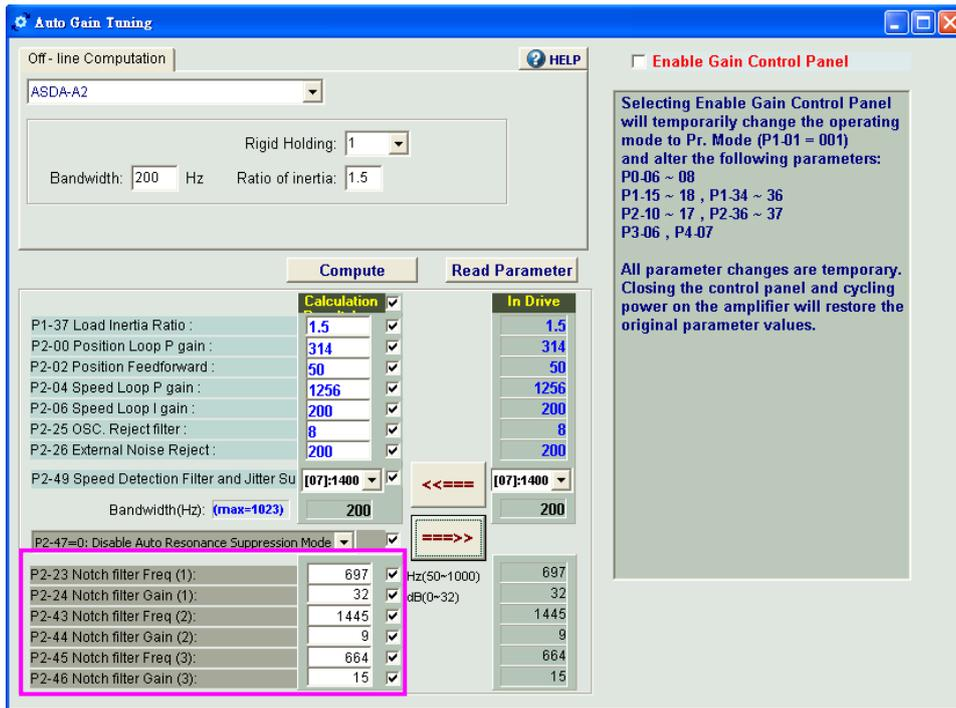
Since we are going to use the third Notch filter, plus the range of the first Notch filter is only 1000 Hz, the following adjustments should be done:
