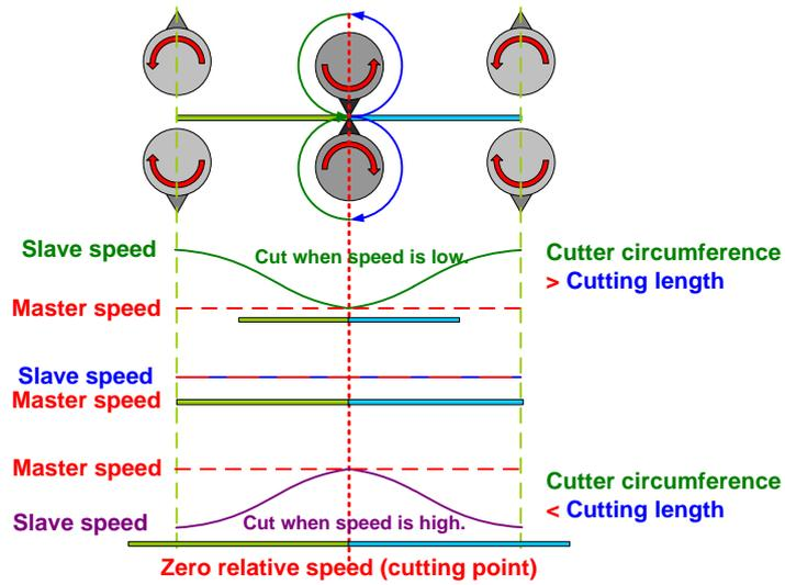
Difference of the speed of slave axis: The operation speed of slave axis can adjust the cutting length. The more constant speed area, the fewer users can do to adjust the cutting length.
