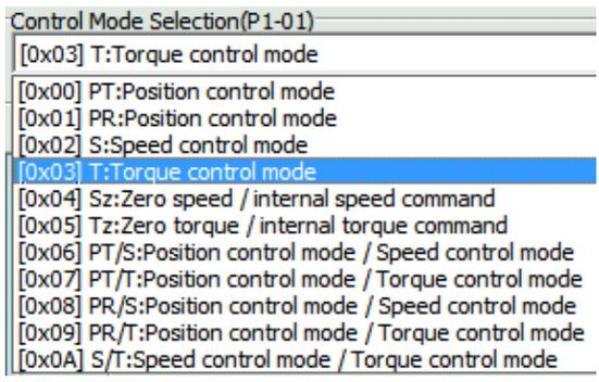
Step 2: Select Torque control mode (T), the setting block on the left will show as below:
