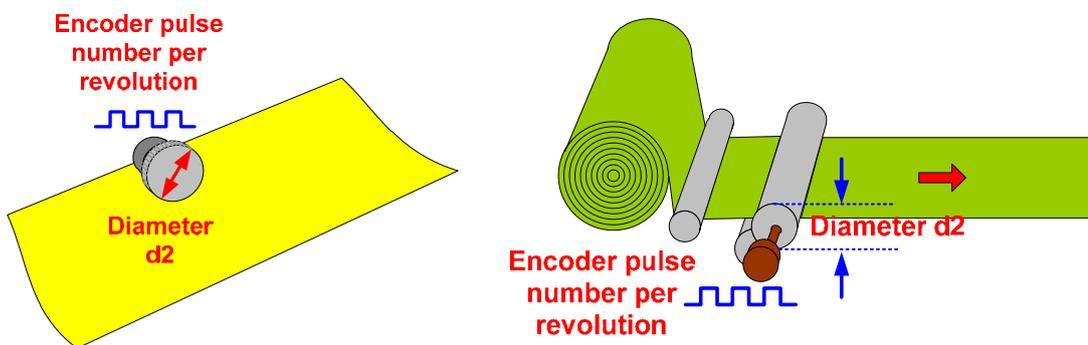
If the pulse number of master axis is already known, then there is no need to enter encoder diameter and resolution of master axis. Check “P5-84 Manually Input” and directly fill in the pulse number in the blank.
