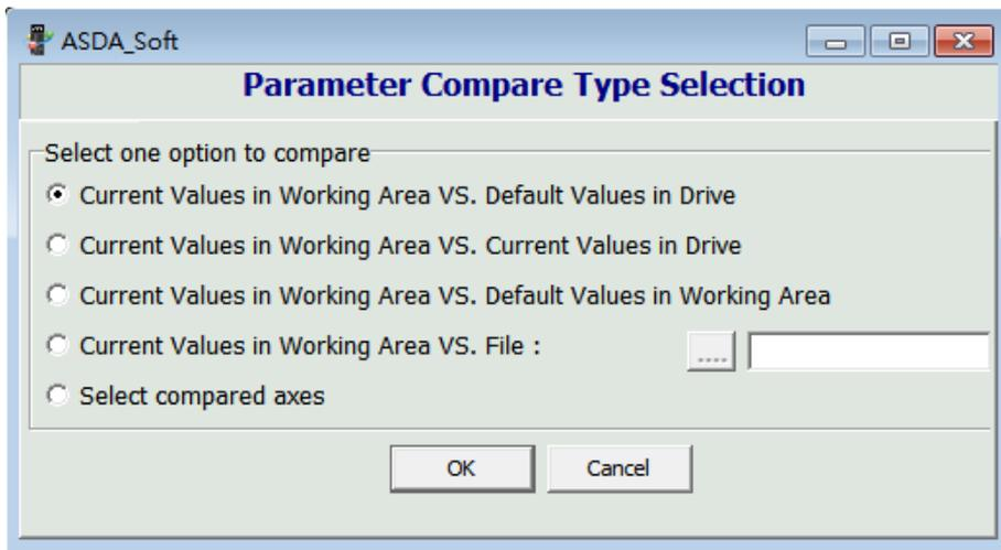
Current Values in Working Area VS. Default Values in Drive: It compares the current value in working area to the default ones in servo drive. Users can compare the difference when the communication is connected.
