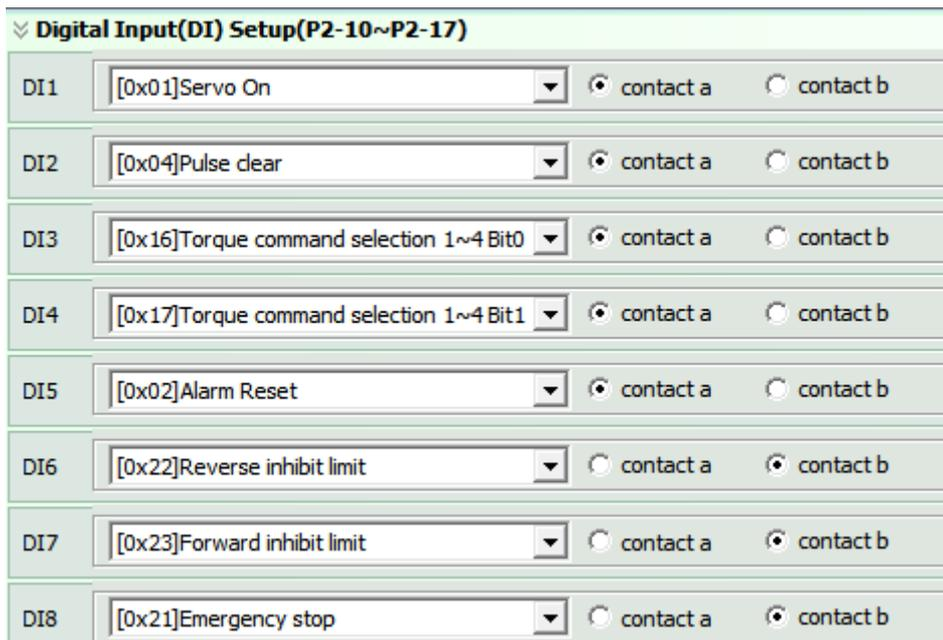
There are 43 command selections of digital input. Users could directly set it up via the drop-down menu.
