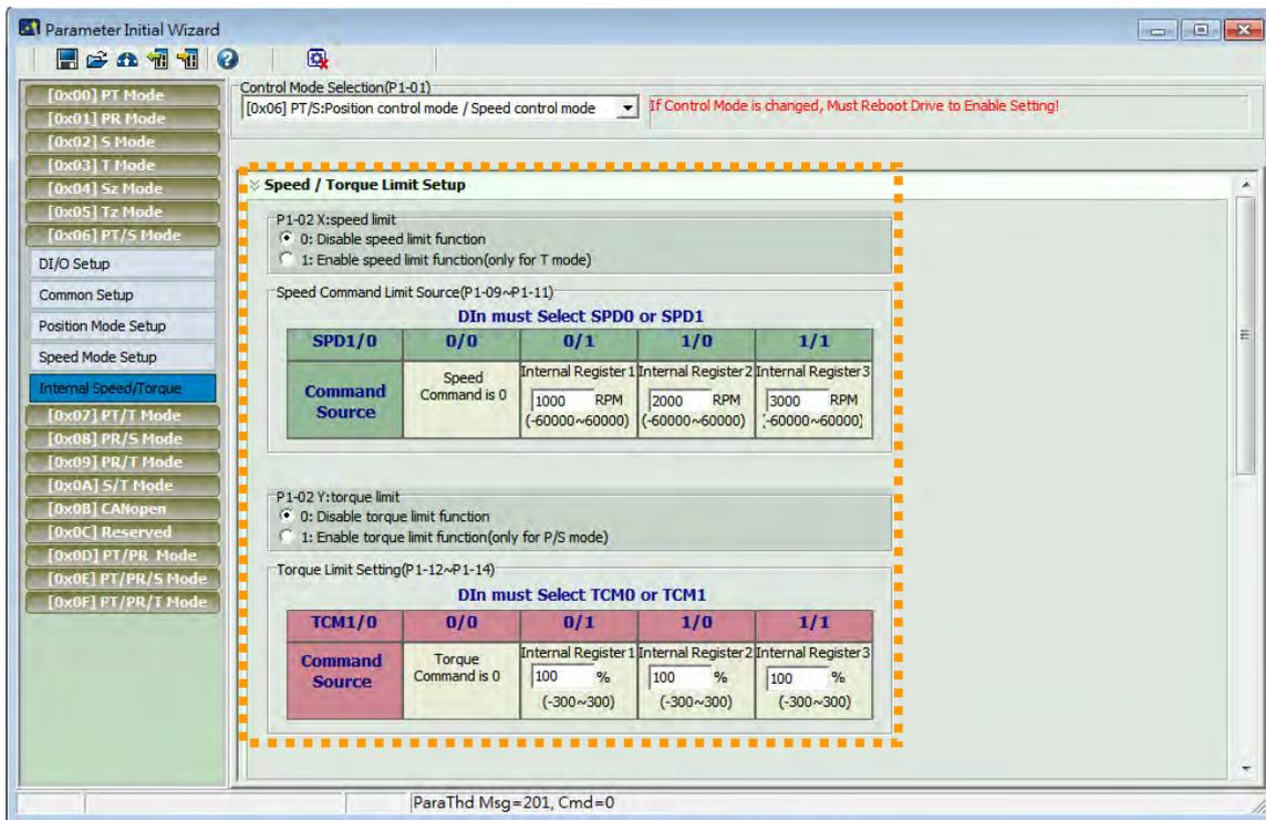
**[0x07] PT/T : Position Control Mode / Torque Control Mode (Dual Mode)**
