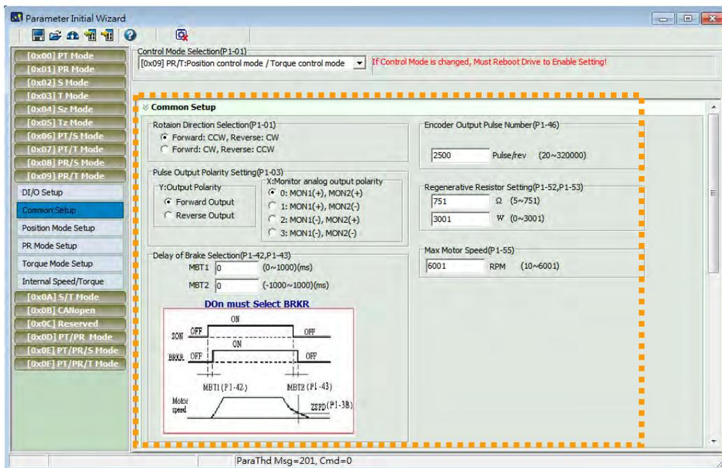
Step 7: Since it is in dual mode, the system provides setting blocks of position (PR) mode, PR mode and torque mode. Setup “Position (PR) Mode” first.
