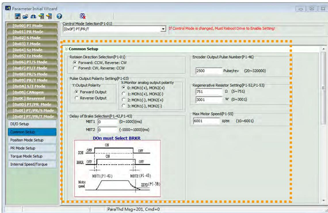
Step 7: Since it is in multi mode, the system provides setting blocks of position (PT) mode, PR mode and torque mode. Setup "Position (PT) Mode" first.
