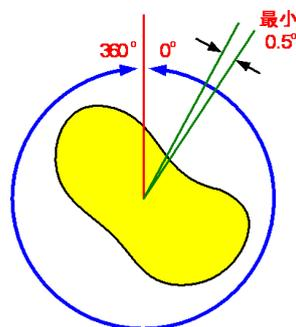
Thus, to create more the sampling points, the E-Cam curve is closer to the actual one. On the contrary, less points brings rougher E-Cam curve. The following steps guide the user to create the E-Cam table.
