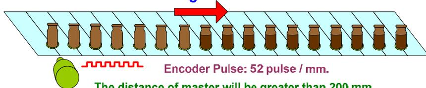
**Step 1:** Enable “E-CAM” and select “Speed Fitting Creation”.
