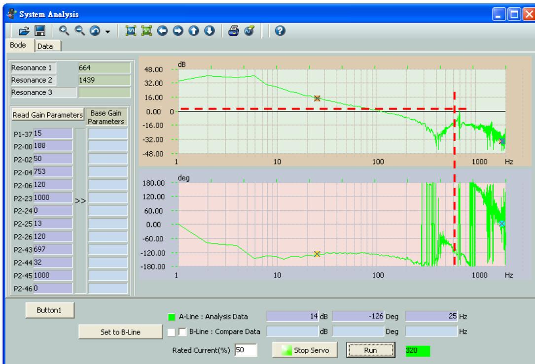
The size of resonance point at 664 Hz is about 3 ~ 4 dB. Thus, adjust Notch filter again.
