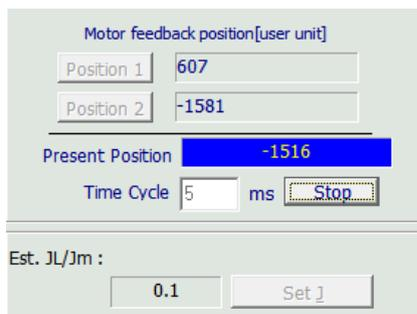
Please observe the variation of inertia ratio. The system will automatically adjust the gain value of control loop. Thus, the inertia ratio will gradually become stable.
