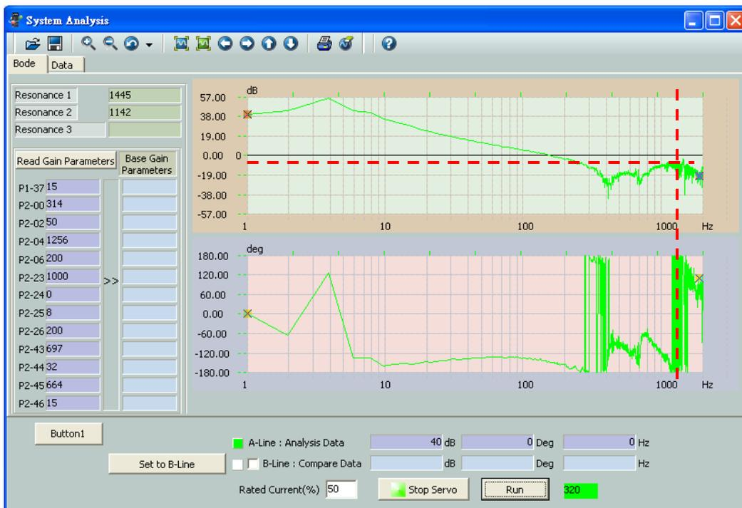
The size of resonance point at 1445 Hz is about -2 dB. Adjust Notch filter again.
