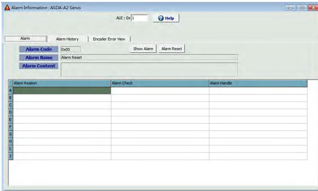
Users can look up alarm messages by entering the alarm number in Off line status. The system will show the alarm description for users' reference.
