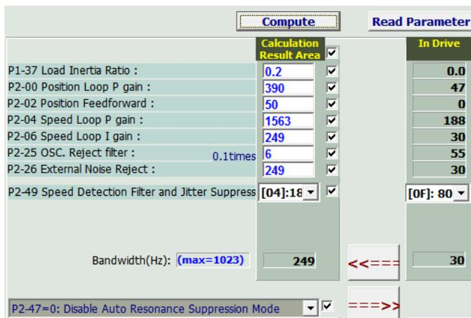
Please pay special attention to the variation of bandwidth. From the above example, the value is adjusted without load, so the bandwidth estimated by the system is 249Hz. However, for general mechanism, high response setting is unnecessary. Users can adjust the bandwidth and gain value according to the real situation.
