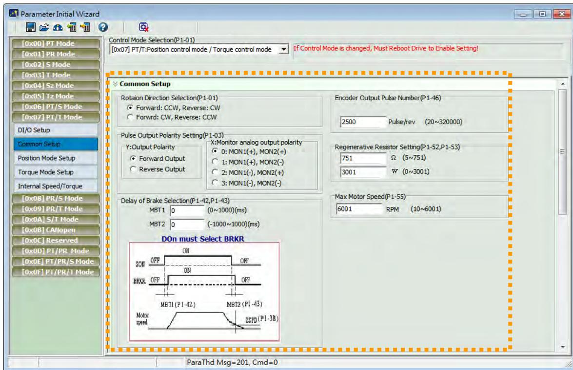
Step 7: Since it is in dual mode, the system provides setting blocks of position (PT) and torque mode. Setup "Position (PT) Mode" first.
