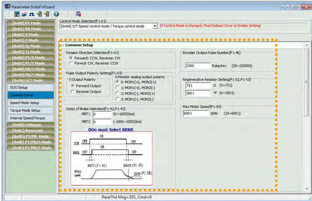
Step 7: Since it is in dual mode, the system provides setting blocks of speed and torque mode. Setup "Speed Mode" first.
