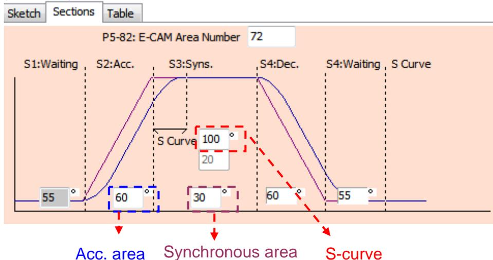
See the above graph as example,  $2 \times 55^\circ$  (waiting area) +  $2 \times 60^\circ$  (Acceleration area) +  $30^\circ$  (Synchronous area) +  $100^\circ$  (S-curve) =  $360^\circ$ .
