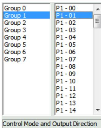
If the user selects P1-01 from Group 1, the below section will display its name, "Input Setting of Control Mode and Control Command".
