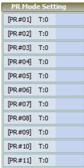
In addition, when users did modify the setting but not download the changed one into the servo drive, the modified area will show the symbol of “\*”.
