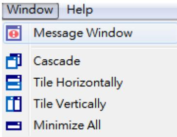
ASDA-Soft provides various selections of window display, such as **【Cascade】**, **【Title Horizontally】**, **【Title Vertically】** and **【Minimize All】**. In addition, **【Message Window】** can display the warning message or fault message of the system when setting up or reading/writing parameters.
