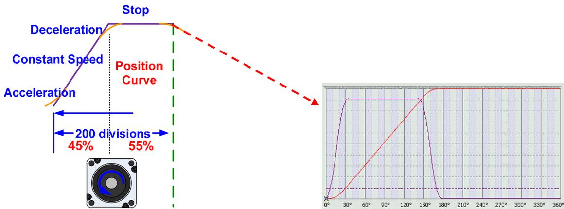
**Export the first section:** Right click the mouse at any column of the E-Cam table. Then, select “Export points”. Since there are 200 parts in this section, users should fill in values between 0 and 200. Save the data when complete.
