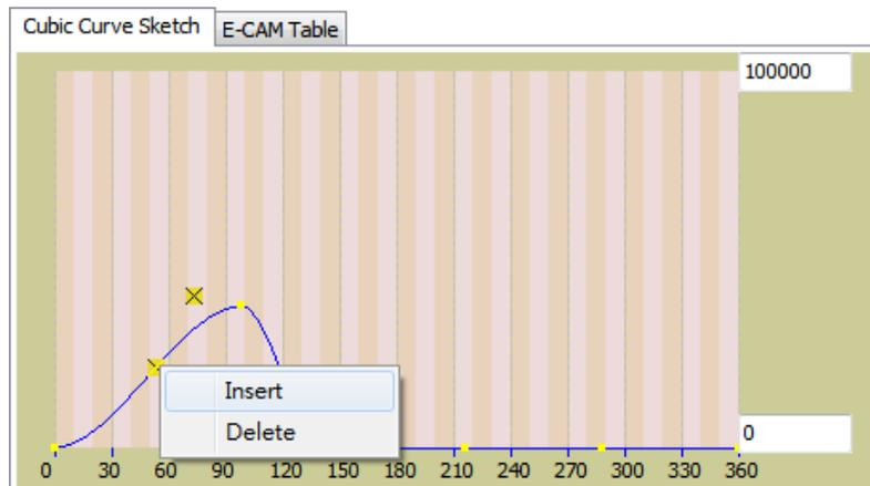
Select "Insert" and the software will add one point around the curve. Since both position and degree of this new point are 0, users have to manually enter these two values and re-program the curve type to create new points.
