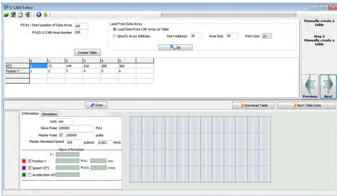
Please note that any type of E-Cam curve can be divided into 720 parts (721 points) at most. The minimum degree of each part in one cycle (360°) is 0.5°.
