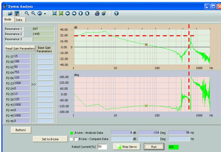
From the result, the size of resonance point at 697 Hz is 32 dB. Adjust the parameter of the first resonance point by this data.
