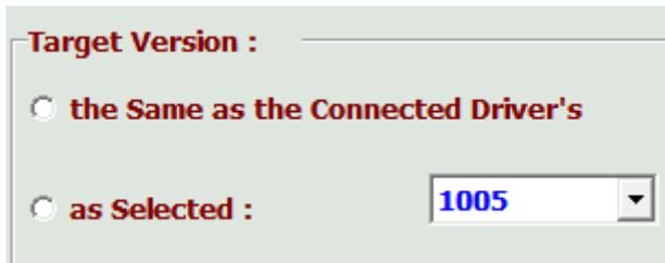
When select **the Same as the Connected Driver's**, regardless the opened firmware version, the system will adjust the parameter value based on the current version.
