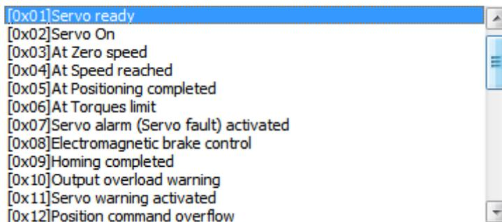
Users can set the digital output (DO) status as “a contact (frequently open)” or “b contact (frequently close)”.
