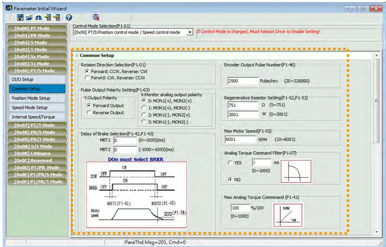
Step 7: Since it is in dual mode, the system provides setting blocks of position (PT) and speed mode. Setup "Position (PT) Mode" first.
