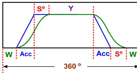
Users have to setup three parameters when using software to setup speed allocation of E-Cam curve: **Acc** (Acceleration area), **Y** (Synchronous area) and **S°** (S-Curve).
