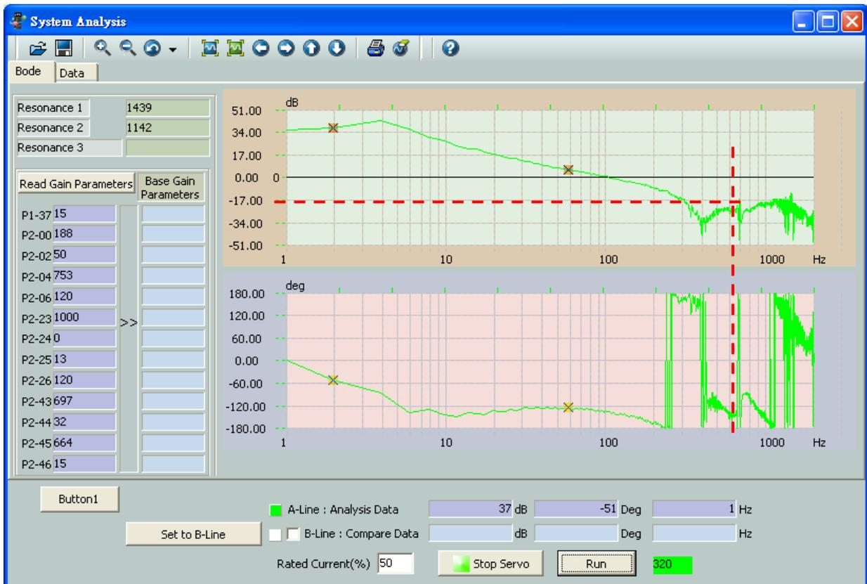
From this graph, the size of resonance point is over 10 dB (about 17 dB). Try to adjust the gain again.
