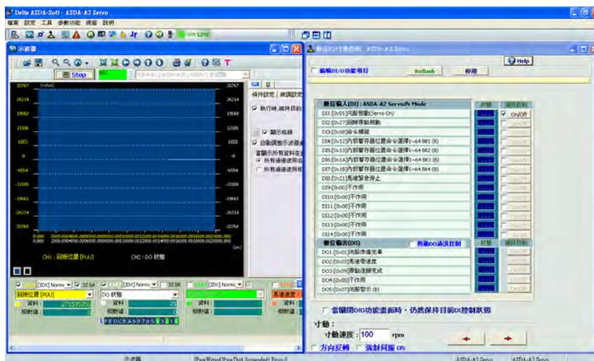
**Step 18:** Take one part of Bold Plot to observe. We can see the triggered cycle of DO4 is 50,131PUU, which is close to 50,000PUU set by us. The length of input length is also close to 100ms of P5-59 CBA.
