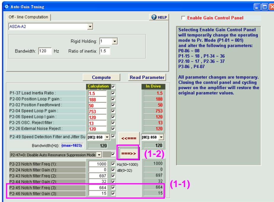
Fill in the resonance frequency and decibel value (dB) to the third Notch filter (P2-45 ~ P2-46).
