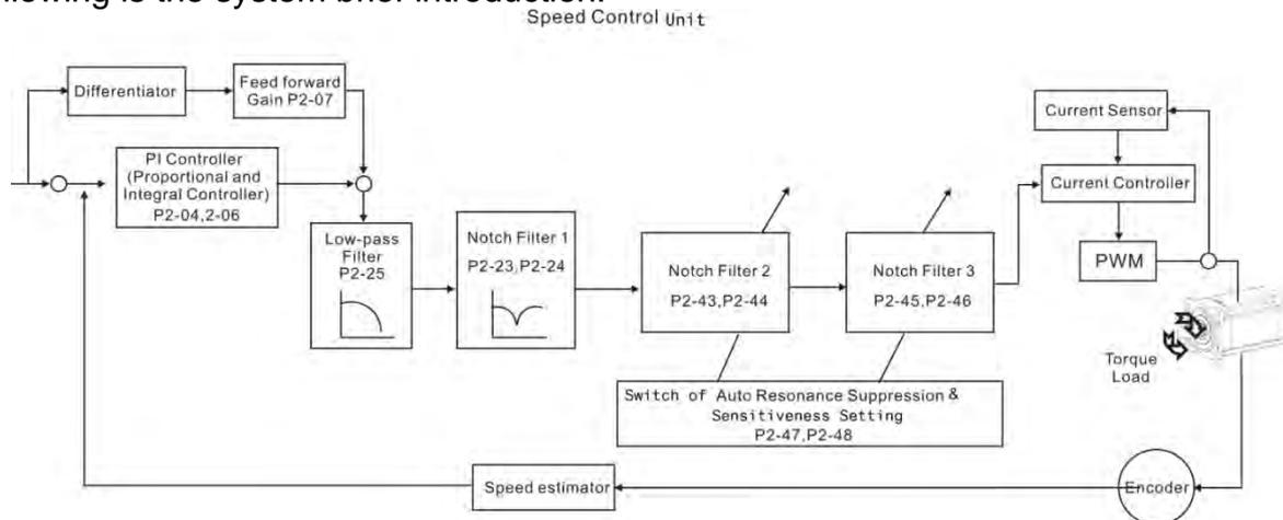
If the resonance frequency is over 2,000Hz, it means the response frequency and gain value have exceeded the one the mechanism can take. It is suggested to reduce both, and then re-do FFT analysis.
