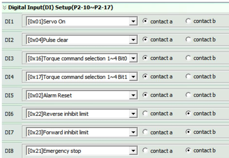
There are 43 command selections of digital input. Users could directly set it up via the drop-down menu.
