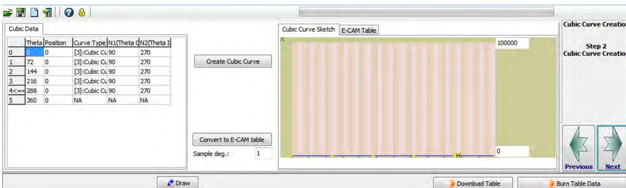
Its setting function is similar to “Manually create a table”. Users can self enter the degree and position of each point.
