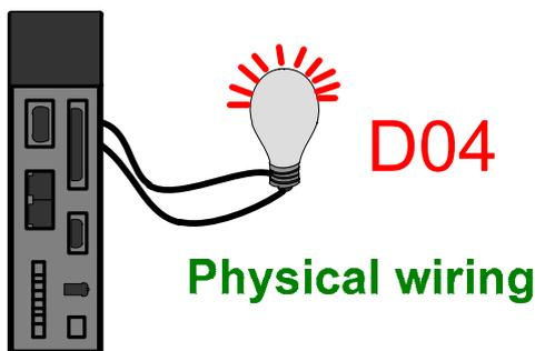
4. Software: Read the output signal from digital IO panel
