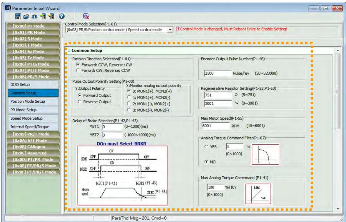
Step 7: Since it is in dual mode, the system provides setting blocks of position (PR) mode, PR mode and speed mode. Setup "Position (PR) Mode" first.
