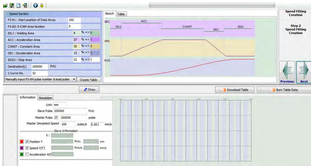
**Step 3:** To create E-Cam curve base on the traveling distance of slave axis. See the following 5 steps.
