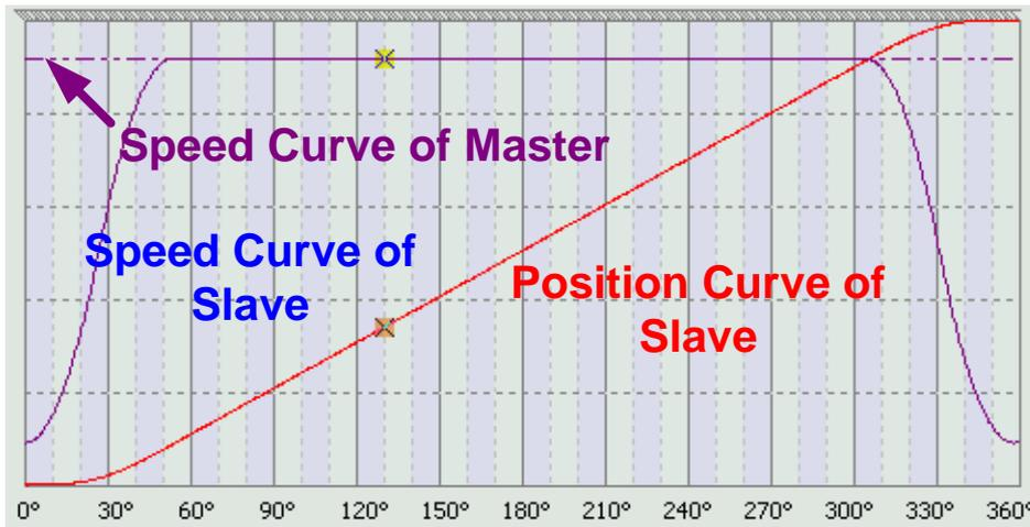
The following three figures illustrate the moving distance of master axis and slave axis as well as the constant speed area: **master axis travels longer distance than slave axis in one cycle.**
