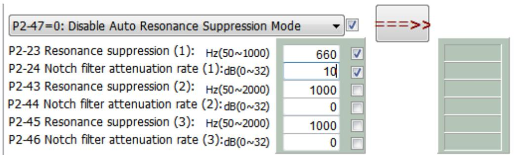
Step 7: Follow the way from above figure to setup parameter (resonance suppression). Then, click
