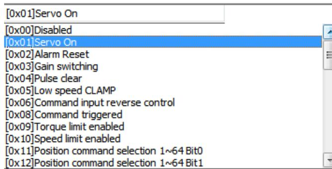
Users can set the digital input (DI) status as “a contact (frequently open)” or “b contact (frequently close)”.
