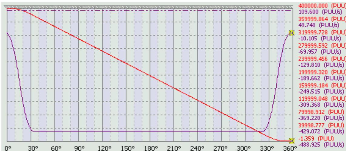
**Export the second section:** Right click the mouse at any column of the E-Cam table. Select “Export points”. Since there are 200 parts in this section, users should fill in values between 0 and 200. Then, save the data of the table.
