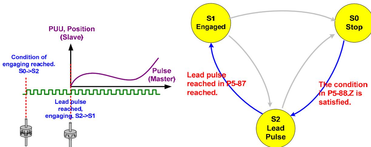
When the engaged condition is established, the E-Cam status will change from stop to pre-engaged, S0 → S2, and start to count the pulse number. When it reaches the pre-engaged amount, the status will change to engaged, S2 → S1.
