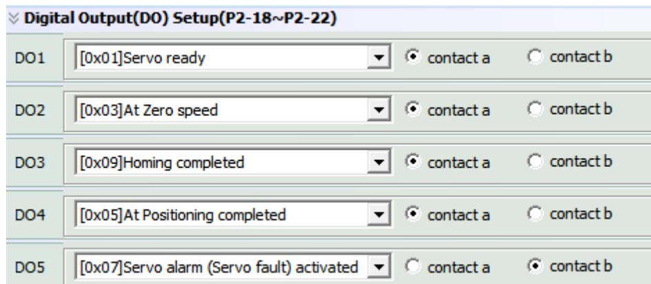
There are 35 command selections of digital output. Users could directly set it up via the drop-down menu.
