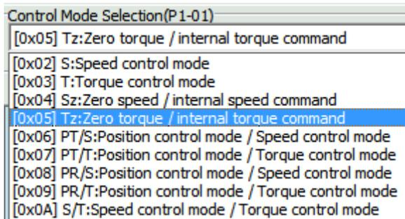
Step 2: Select Zero torque control mode (Tz), the setting block on the left will show as below:
