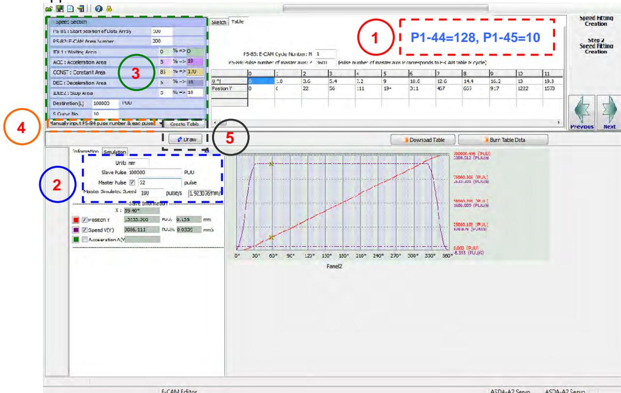
The table filling steps in this example is almost the same as the above description. The difference is on Step 4 when selecting **Based on P5-84 pulse number, calculate lead pu**.
