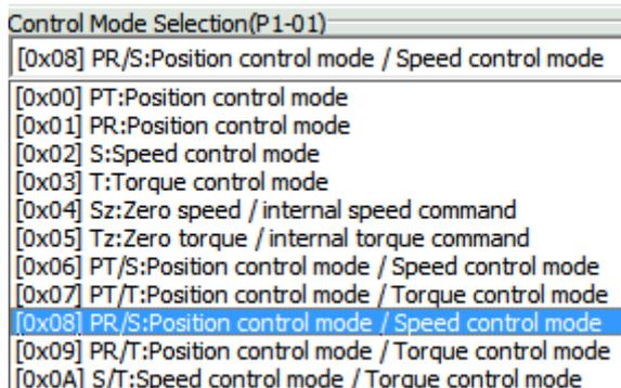
Step 2: Select position control mode / speed control mode, the setting block on the left will show as below:
