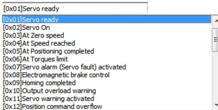
Users can set the digital output (DO) status as “a contact (frequently open)” or “b contact (frequently close)”.
