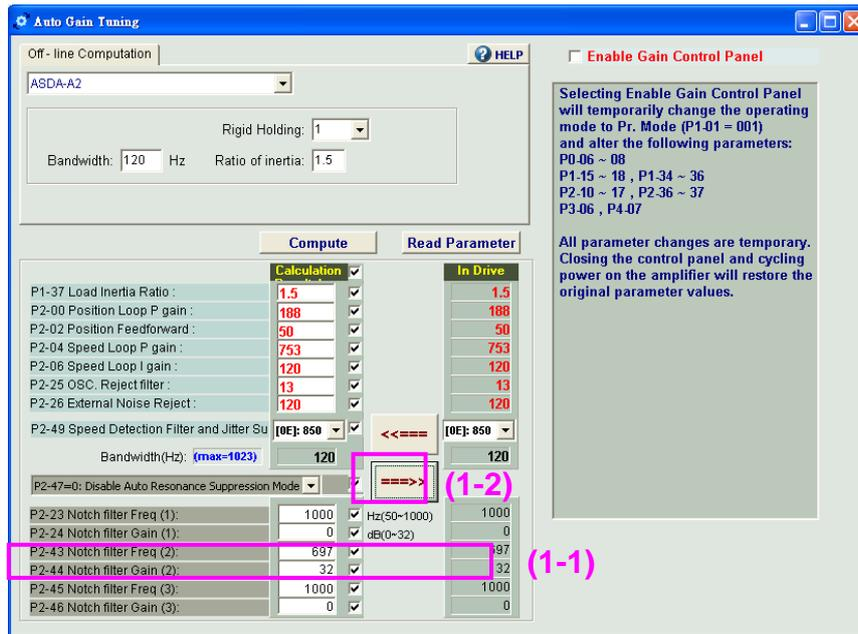
Fill in the resonance frequency and decibel value (dB) to the second Notch filter (P2-43 ~ P2-44).
