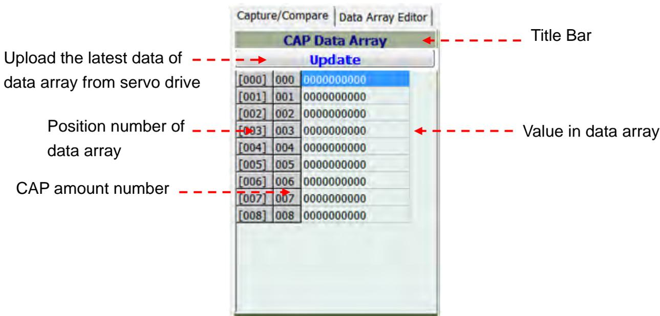
During the test process, users can click **Update** to update the value in data array if needed.
