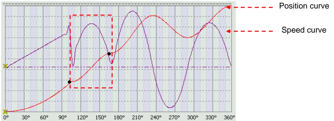
Adjust the curve from the second to third point as "linear". Users can see the speed curve between two points becomes linear, which causes dramatic change.
