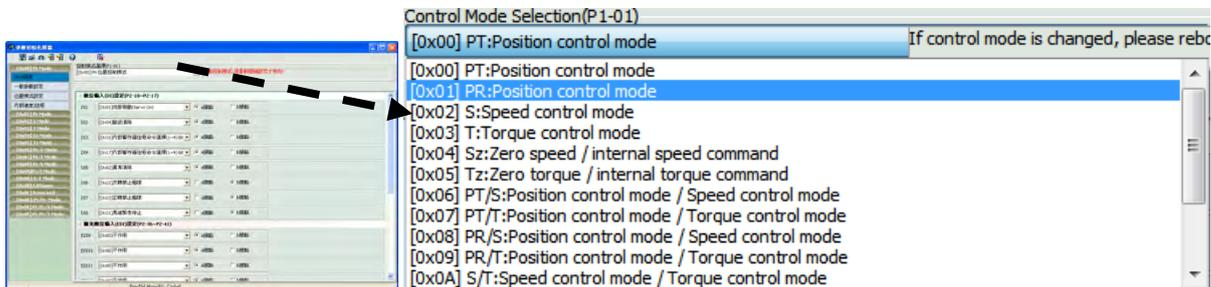
Use drop-down list to setup -- [0x04] Sz: Zero speed / internal speed command
