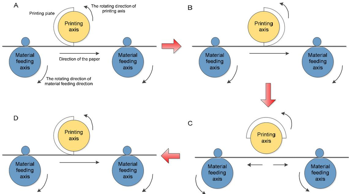
ASDA-Soft provides servo setting wizard for intermittent motion control. Users could plan it according to the required print area and blank area and manually adjust the angle in synchronous area and waiting area. Complete the setting of material feeding axis by following the steps below.
