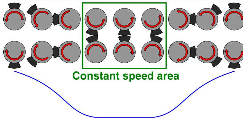
From the above figure, constant speed area is determined by material. E-Cam curve shall be set according to the material.
