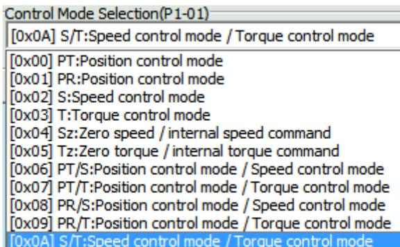
Step 2: Select Speed control mode / Torque control mode, the setting block on the left will show as below:
