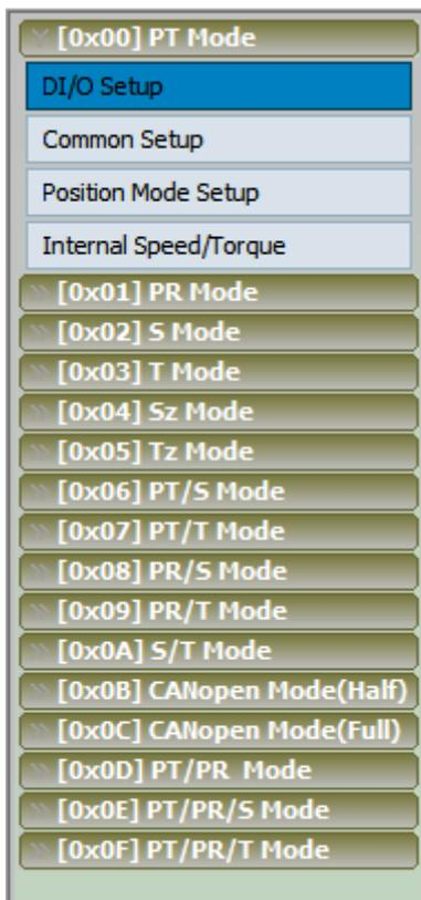
**[Function Setting]** : Users can setup parameters and functions of each control mode in this page.
