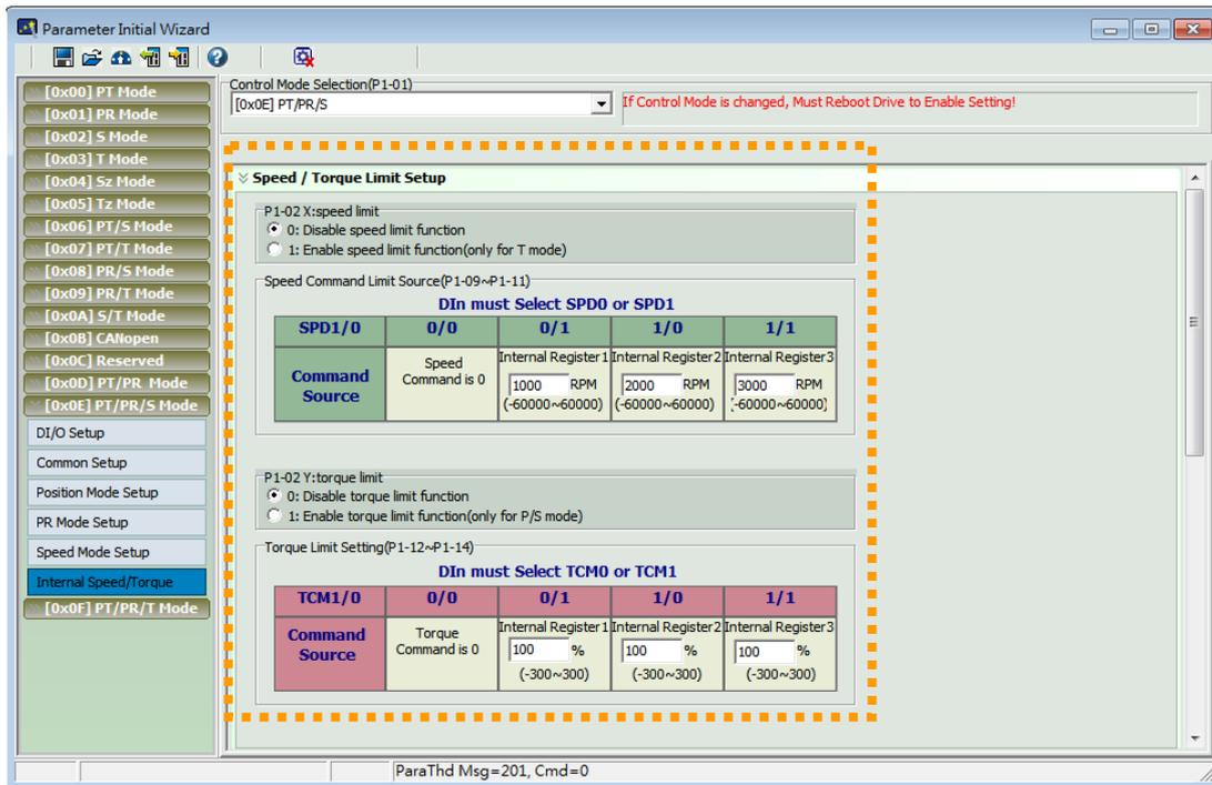
**[0x0F] PT/PR/T : Multi Control Mode (Position and Torque Mode)**
