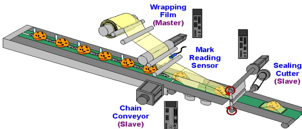
Synchronous axis has the function of mark tracking in packing machine. When the cutting is inaccurate, the system will correct the cutting timing so as to adjust the cutting length and position.
