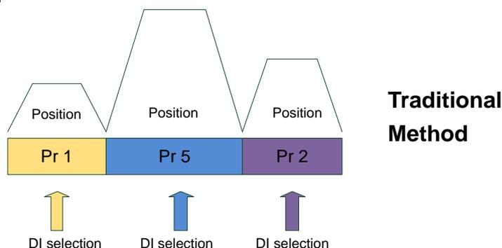
Innovative Method of ASDA-A2: The command can be changed by external trigger or internal interruption. Various external triggering methods are offered in ASDA-A2, which differs from the traditional one. Users can operate with different kind of functions, such as homing control, position control, speed control, procedure jump, parameters written-in and ect.
