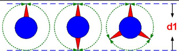
**Pulse number and encoder diameter:** Encoder diameter is mechanism that rotates along with the material feeding. Its resolution should be a known parameter.
