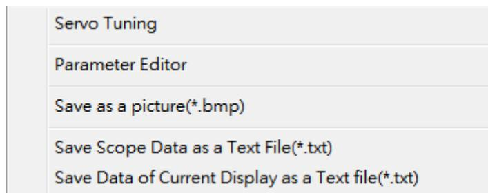
**【Servo Tuning】** : Click to enable the function of “Auto Gain Tuning”.
