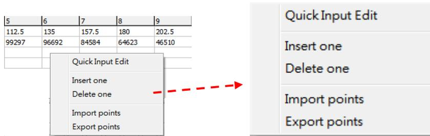
This enables users to edit E-Cam table in a very quick and easy way. For example, users can copy one same section of E-Cam curve or insert / delete one point in E-Cam curve that just created.
