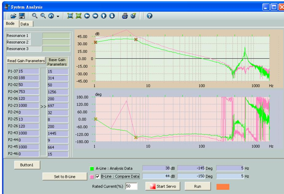
A-Line: Before gain tuning; B-Line: After gain tuning.
