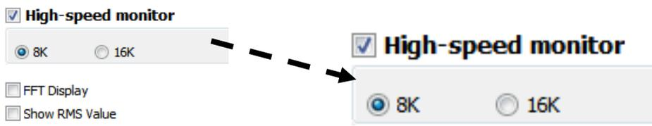
Its initial setting is 8k Hz, if check 16k Hz, channel 2 and 4 will be closed automatically. This is because the system has to share the bandwidth to channel 1 and 3.
