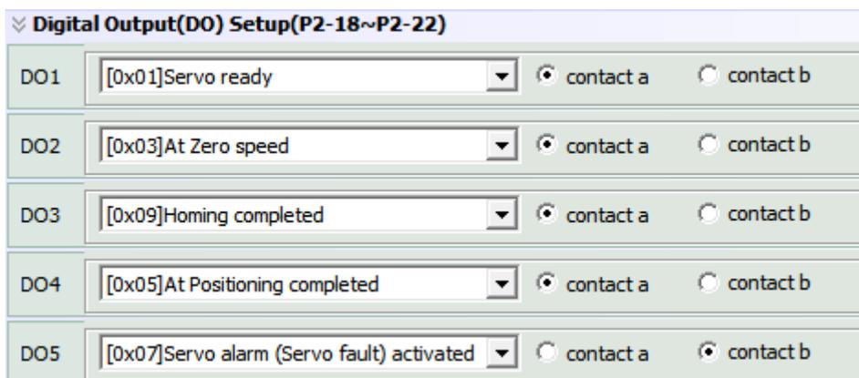
There are 35 command selections of digital output. Users could directly set it up via the drop-down menu.
