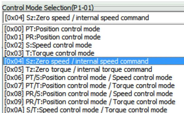
Step 2: Select Zero speed control mode (Sz), the setting block on the left will show as below:
