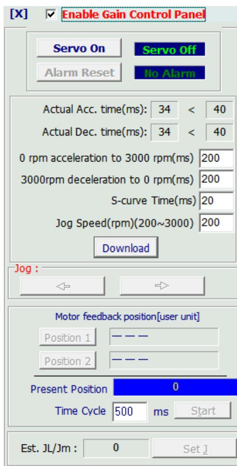
Step 2: Setup the parameter of motor speed. It is suggested to set from low speed to the actual operation one:
