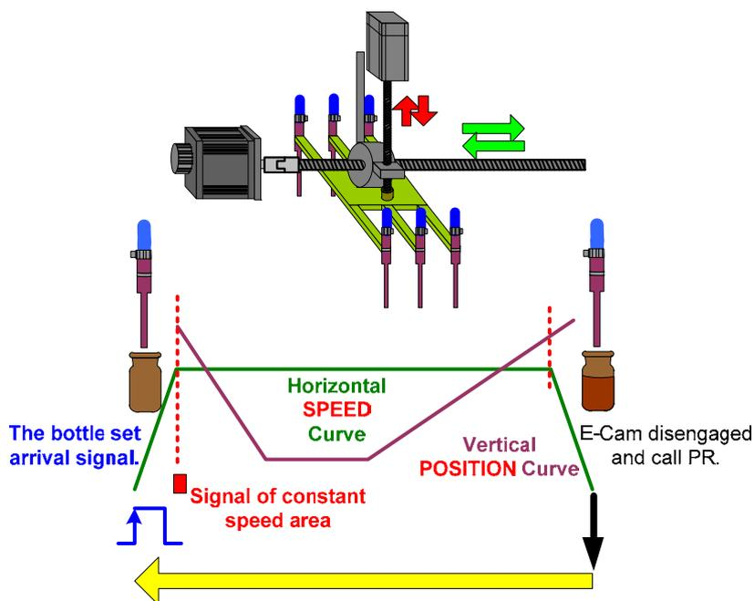
This system has two E-Cam curves. One is for controlling the platform in horizontal direction and another one is for controlling the filling axis in vertical direction. A complete cycle starts when the bottle is in accurate position and activate the signal, then ends when the platform returning to the start position controlled by PR command.
