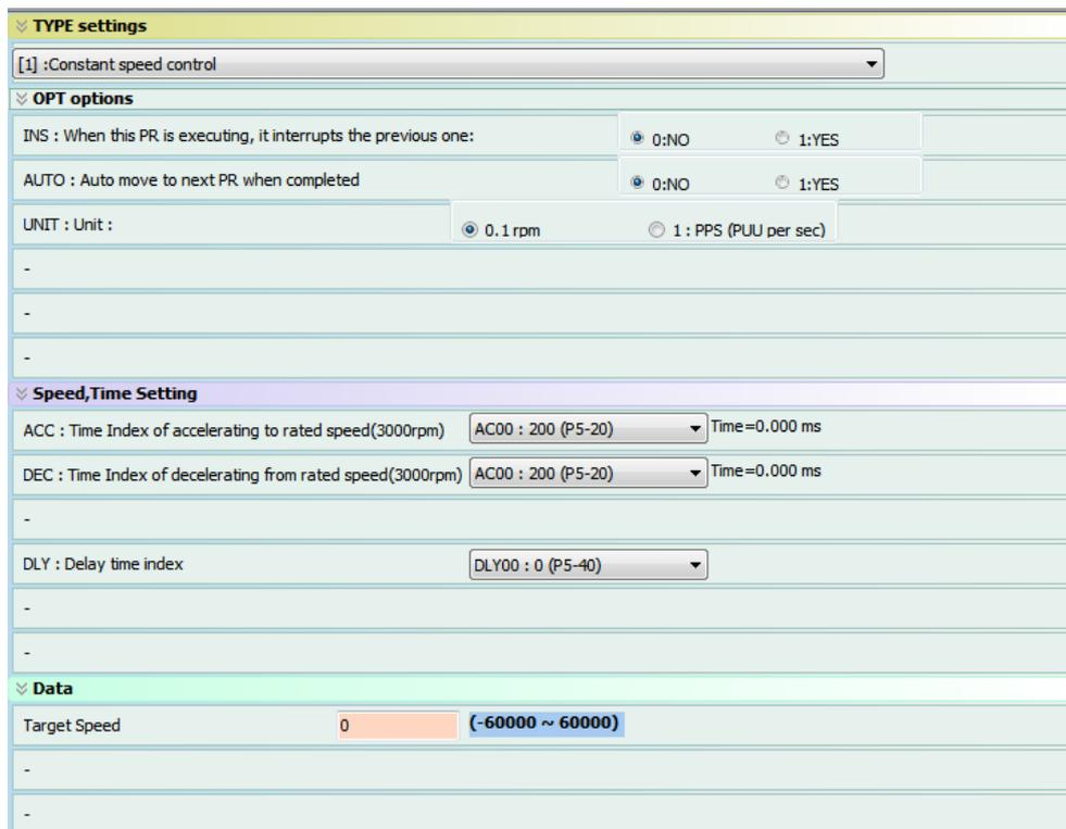
**OPT options** : In constant speed control, 3 parameters can be used to interrupt PR
