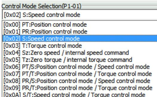
Step 2: Select Speed control mode (S), the setting block on the left will show as below:
