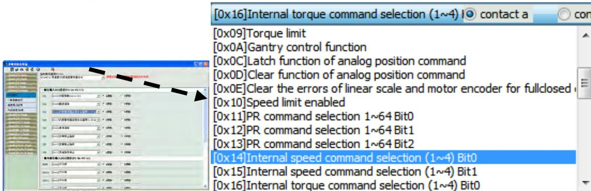
Use drop-down list for setting -- [0x14] Speed command selection (1~4) Bit0
