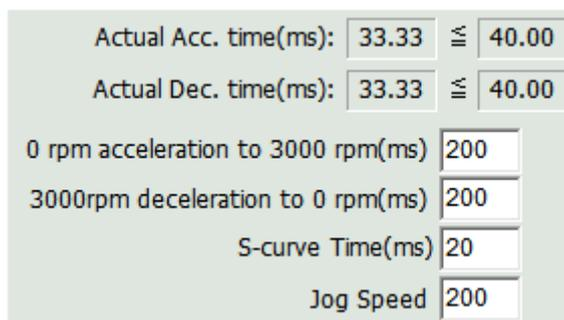
Take the above figure as the example. When the acceleration time and deceleration time is 200ms; the setting value should be:
