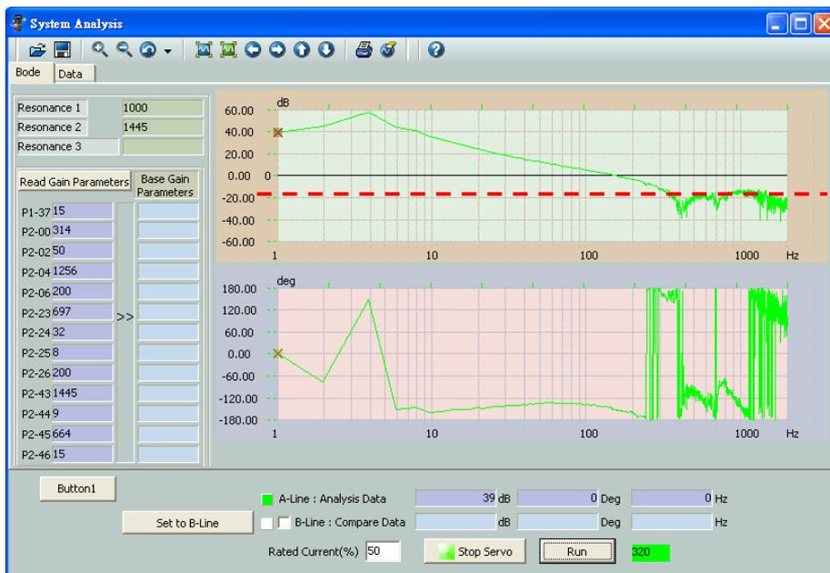
Step 11: Compare the data of A-Line and B-Line. The red curve is newly adjusted and the green one is the original one after the first gain setting. Apply the function of system analysis to suppress resonance point and adjust the system until it is stable.
