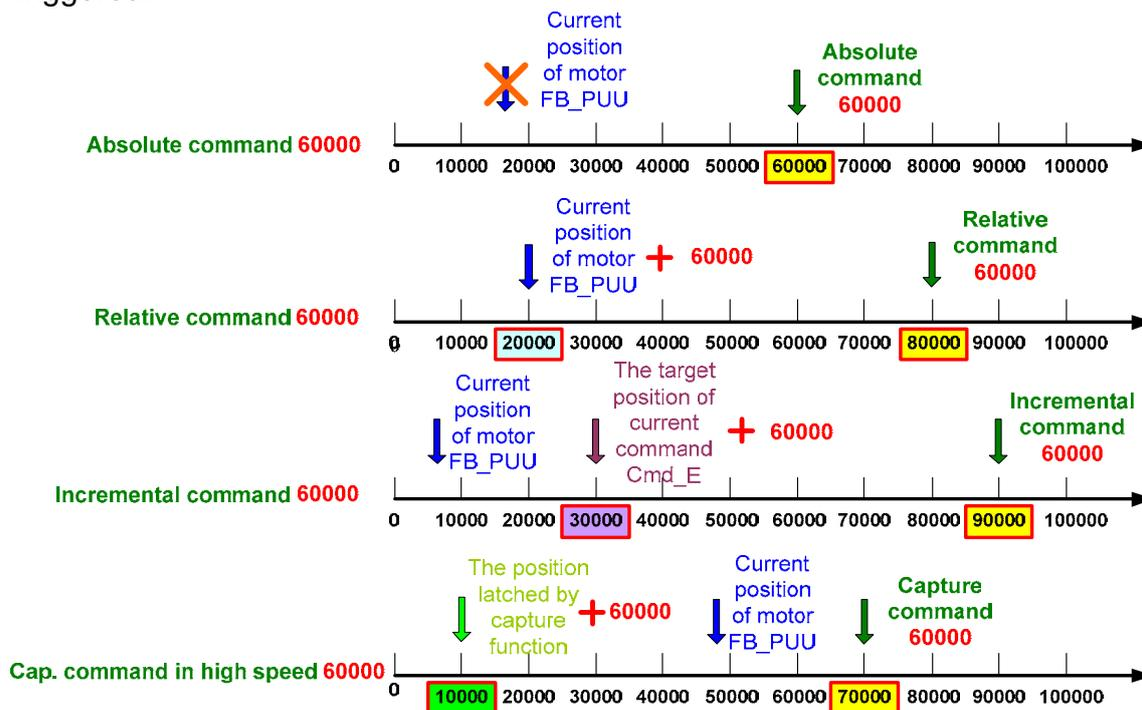
Setup motion control first and then determine the PR command. It means to define the acceleration, deceleration and target speed of the motor. Without the setting of interrupt (INS) and overlap command (OVLP), the delay time starts when target position is reached.
