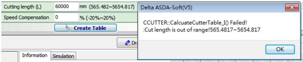
Please pay special attention to the **curve limit** set by the software. It is for avoiding the unreasonable rotary shear curve. For instance, if cutting length A is much shorter than the moving distance a of slave axis when cutting, it will be unable to increase the speed of slave axis to satisfy the demand of short cutting length. If the value of R is too small, it might need to modify the mechanism to conquer the problem.
