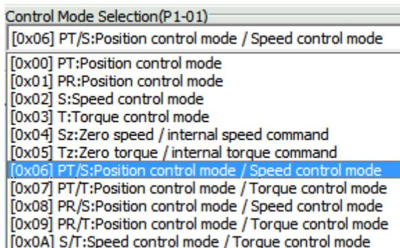
Step 2: Select Position control mode / Speed control mode, the setting block on the left will show as below:
