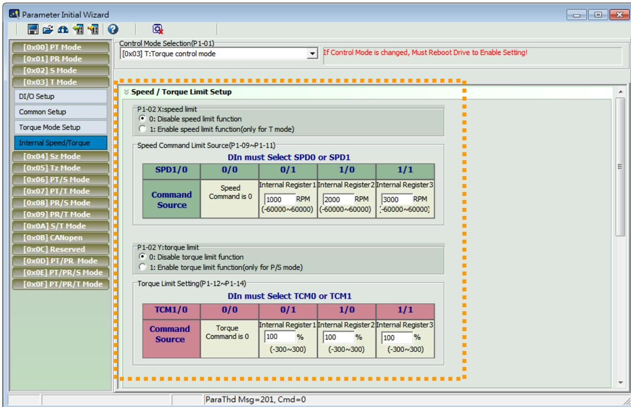
**[0x04] Sz : Zero Speed / Internal Speed Command**
