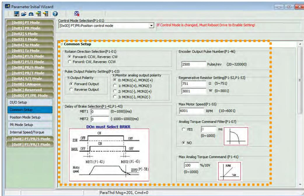
Step 7: Since it is in dual mode, the system provides setting blocks of position (PT) and PR mode. Setup "Position (PT) Mode" first.
