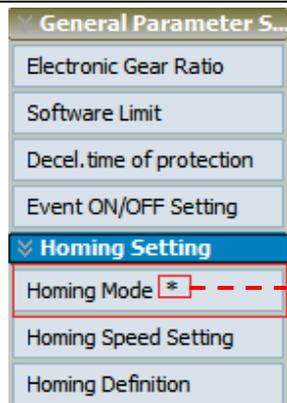
It means the setting is modified but hasn't been downloaded into the servo drive.
