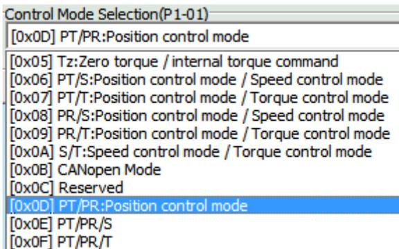
Step 2: Select dual position control mode. The setting block on the left will show as below:
