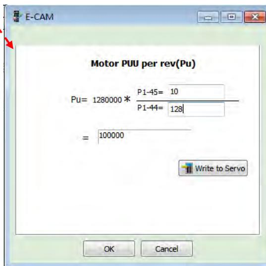
**Cutting length (L):** Cutting length of the material. Please enter the desired value.
