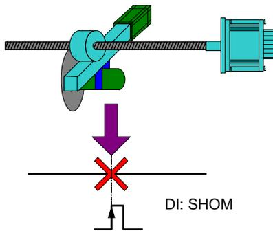
The home position is defined to the place the motor stops at the moment of SHOM signal triggered.
