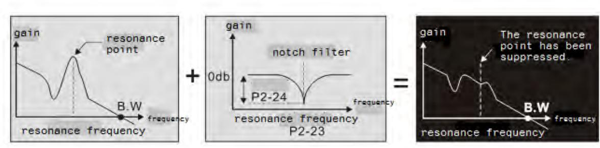
Step 6: The resonance point is at 660Hz, the relative value is 10, 000.
