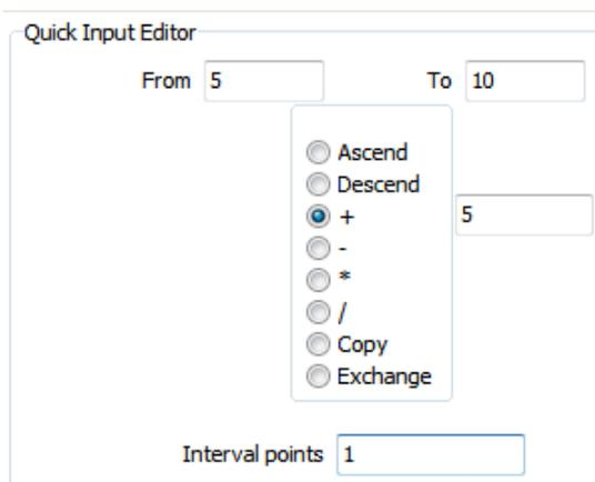
Setup the position of E-Cam point, 5 to 10. Each point plus 5 and the interval value is 1:
