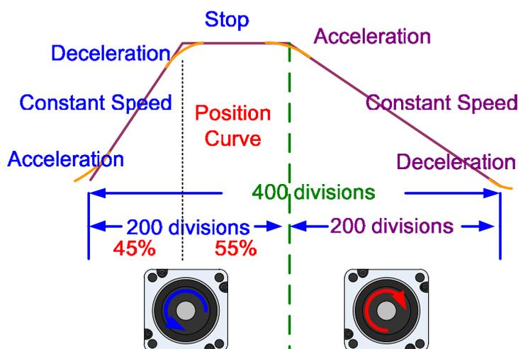
This method is to create the curve by dividing the same rotating direction of curves into different sections. The setting method will be elaborated in "Speed Fitting Creation".
