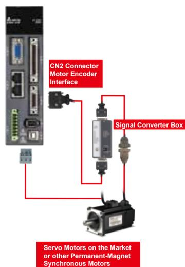
3. When not using Delta's servo motor and if the encoder signals are square wave, the square wave can be converted into communication signals directly through the CN5 connector for the use of Delta's ASDA-A2R servo system.
