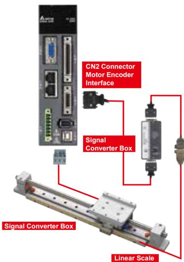
5. When using the linear motor with a linear scale and if the encoder signals are square wave, the square wave can be converted into communication signals directly through the CN5 connector for the use of Delta's ASDA-A2R servo system. In addition, when a Hall Sensor is included and placed in-between, the signal can be transmitted via CN5 connector and controlled.
