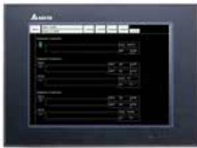
Built-in PLC ladder monitor devices allow users to display programs in real time and confirm machine operations without using a PC.
