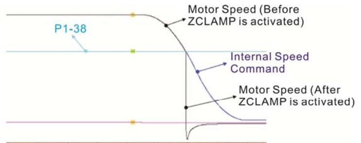
Bit10 = 1: The command source is analog speed command. ZCLAMP function will use the analog speed command without acceleration / deceleration processing to judge if this function is enabled. When ZCALMP conditions are established, the motor speed decelerates to 0 through S-curve. If not, the motor follow the analog speed command through S-curve.
