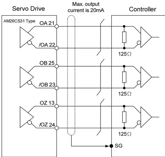
**C14: Encoder signal output (Opto-isolator)**
