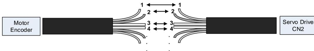
If not using housing and directly wire the cores, please follow the corresponding core number for wiring. For example, core number 1 from the servo drive CN2 should connect to core number 1 from the motor encoder; core number 2 from the servo drive CN2 should connect to core number 2 from the motor encoder and so on. Please number the cores from the servo drive in order and then connect it to the encoder.
