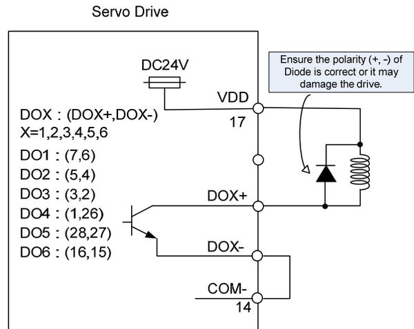
**C7:** Wiring of DO signal. The servo drive applies to the external power and the resistor is general load.
