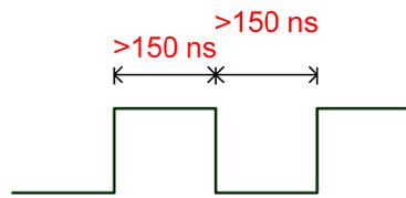
When the pulse frequencies of high-level duty and low-level duty both are greater than 150 ns, the signal will not be filtered (that is, the pulse command will pass through).
