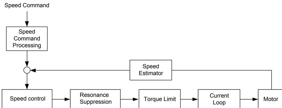
The speed command unit is to select speed command source according to Section 6.3.1, including the scaling (P1-40) setting and S-curve setting. The speed control unit manages the gain parameters of the servo drive and calculates the current command for servo motor in time. The resonance suppression unit is to suppress the resonance of mechanism. Detailed descriptions are shown as the following:
