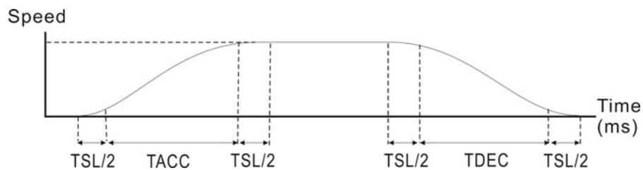
P1-34: Set the acceleration time of acceleration / deceleration of trapezoid-curve
