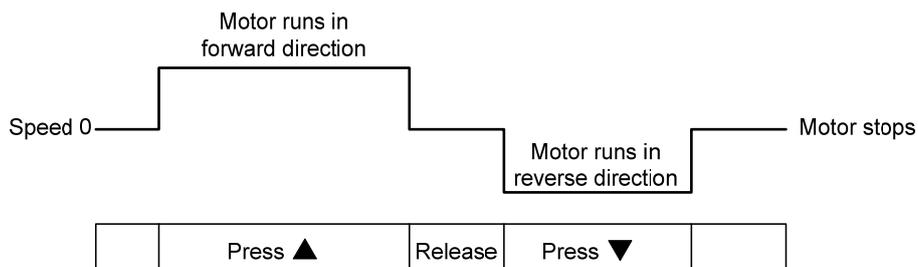
If the motor does not run, please check if the wiring between UVW and encoder cable is correct.
