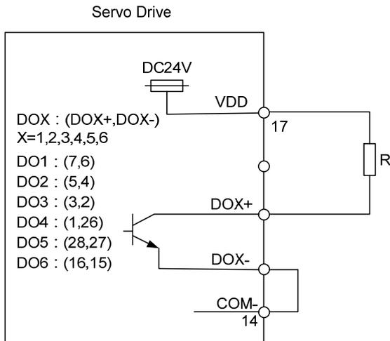
**C6:** Wiring of DO signal. The servo drive applies to the internal power and the resistor is inductive load.
