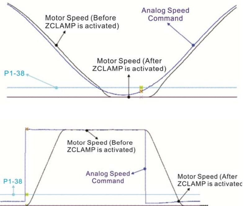
Bit10 = 1: The command source is register. ZCLAMP function will use the register with acceleration / deceleration processing to judge if this function is enabled. When ZCLAMP conditions are established, the motor speed will be set to 0.
