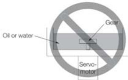
4. Do not use the servo motor in an environment with cutting fluid. Depending on the type of cutting fluid, the sealing material, the coated colloids, cables, or other components may be affected or even deteriorate.
