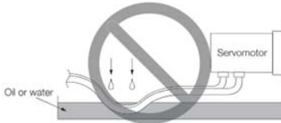
2. If oil or water is unavoidable, please use oil-resistant cables. Delta does not provide oil-resistant cables.
