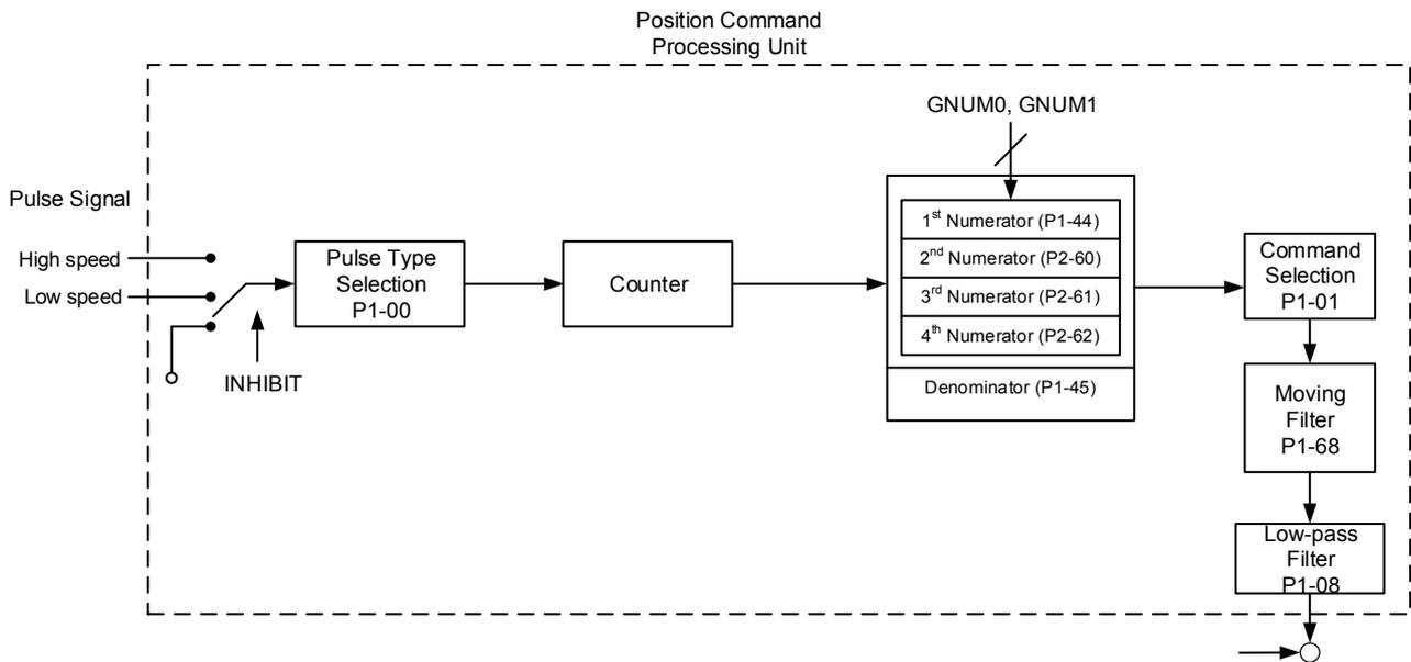
PT mode which is shown in the figure can be selected via P1-01. It can set E-gear ratio for the proper position resolution. Moreover, either S-curve filter or low-pass filter can be used to smooth the command. See the description in later parts.
