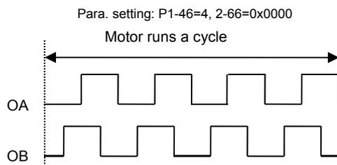
1: 0x8000. The setting value of P1-46 is the pulse number of quadrupler frequency per cycle.
