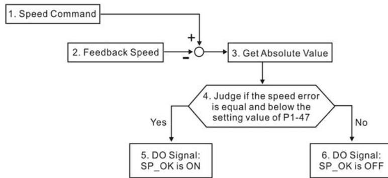
1. Speed Command: It is the command issued by the user (without acceleration / deceleration), not the one of front end speed circuit.
