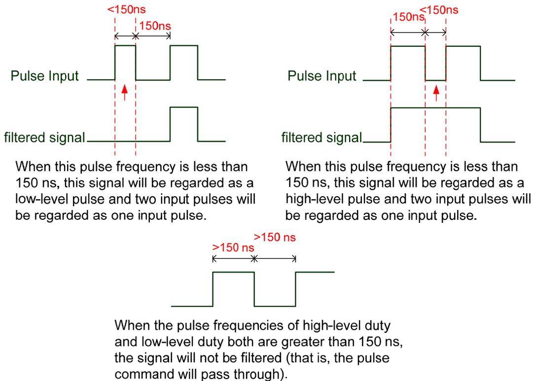
If the user uses 2 ~ 4 MHz input pulse, it is suggested to set the filter value to 4.
