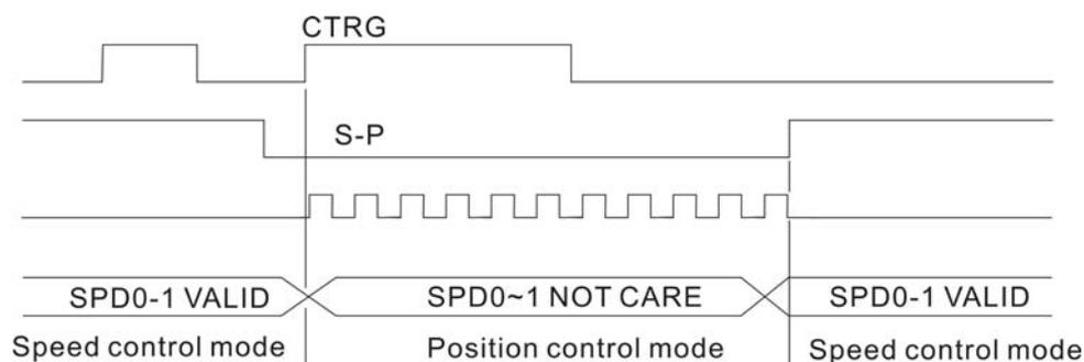
Figure 1. : Speed / Position Control Mode Selection
