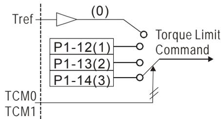
Users could use torque limit function via parameter setting or DI triggering. That is to say, set P1-02 to 0x0010 or trigger DI will do. Also, users could enable or disable the limit function via DI.TRQLM, which is a more flexible way but would need to take one DI setting. Torque limit can be enabled by P1-02 or DI. DI.TCM0 and DI.TCM1 are for selecting the limiting source.
