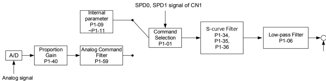
The upper path is the command from register while the lower one is external analog command. The command is selected according to the status of SPD0, SPD1 and P1-01 (S or Sz). Usually, S-curve and low-pass filter are applied for having a smooth resonance of command.
