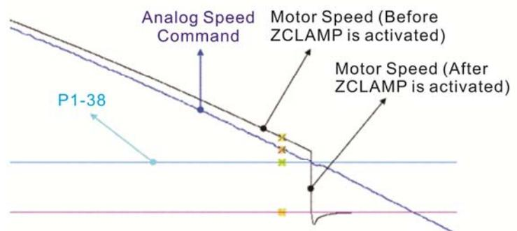
Bit10 = 0: The command source is register. ZCLAMP function will use the register speed command with acceleration / deceleration processing to judge if this function is enabled. The motor will be locked at the position where ZCALMP conditions are established.
