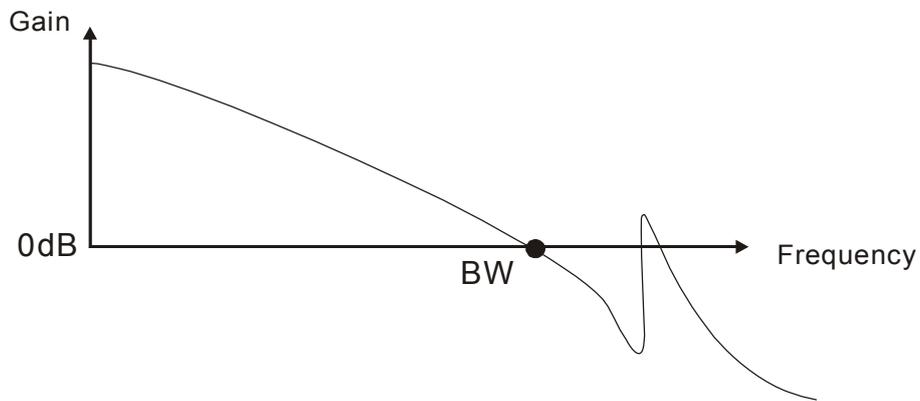
If users know the resonance frequency, notch filter (parameter P2-23 and P2-24) can directly eliminate the resonance. The frequency setting range of notch filter is merely from 50 to 1000 Hz. The suppression strength is from 0 to 32 dB. If the resonance frequency is not within the range, it is suggested to use low-pass filter (parameter P2-25).
