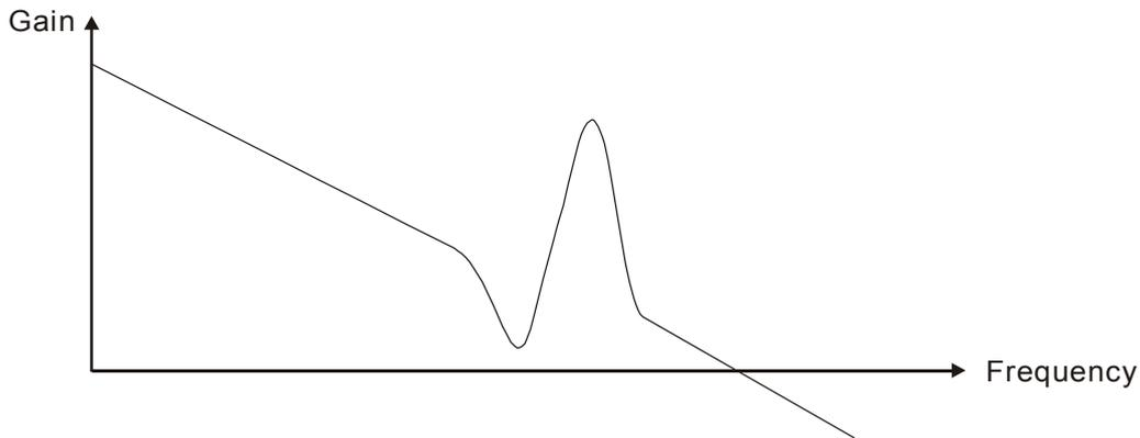
When the value of P2-25 is increased from 0, BW becomes smaller (See as the following diagram). Although it solves the problem of resonance frequency, the response bandwidth and phase margin is reduced.
