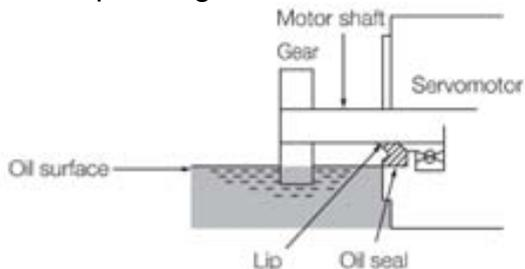
2. The oil seal cannot be submerged in the liquid; it can only withstand splashes of oil.
