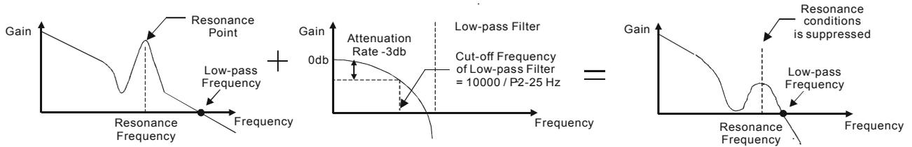
When the value of P2-25 is increased from 0, BW becomes smaller. Although it solves the problem of resonance frequency, the response bandwidth and phase margin is reduced. Also, the system becomes unstable.
