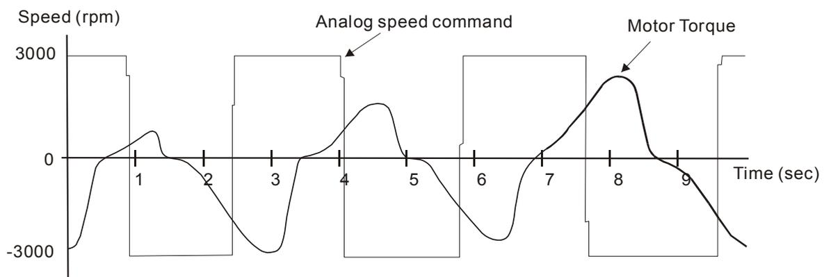
Analog speed command filter smooth the analog input command. Its time program is the same as S-curve filter in normal speed. Also, the speed curve and the acceleration curve are both continuous. The above is the diagram of analog speed command filter. The slope of speed command in acceleration and deceleration is different. Users could adjust the time setting (P1-34, P1-35, and P1-36) according to the actual situation to improve the performance.
