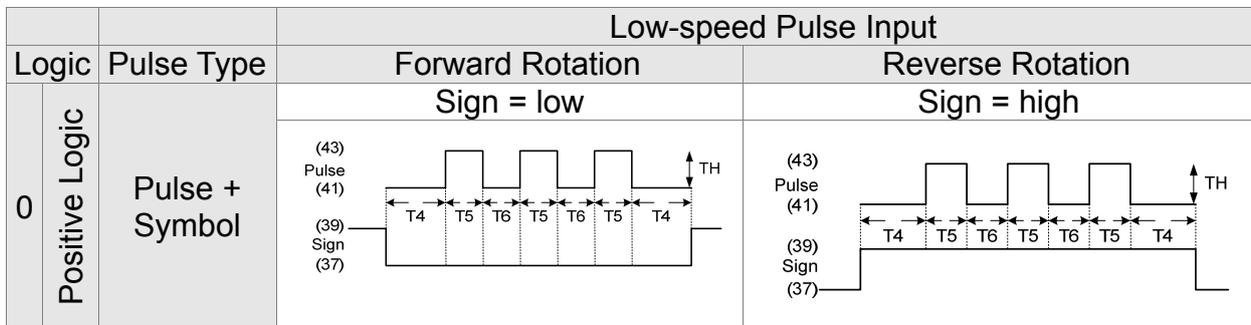
Digital circuits use 0 and 1 to represent the high and low voltage levels. In positive logic, 1 represents high voltage and 0 represents low voltage; in negative logic, 1 represents low voltage and 0 represents high voltage.
