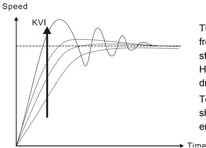
The bigger KVI value cause greater low-frequency gain and shorten the time the steady-state error returns to zero. However, the phase margin will dramatically decrease as well.
