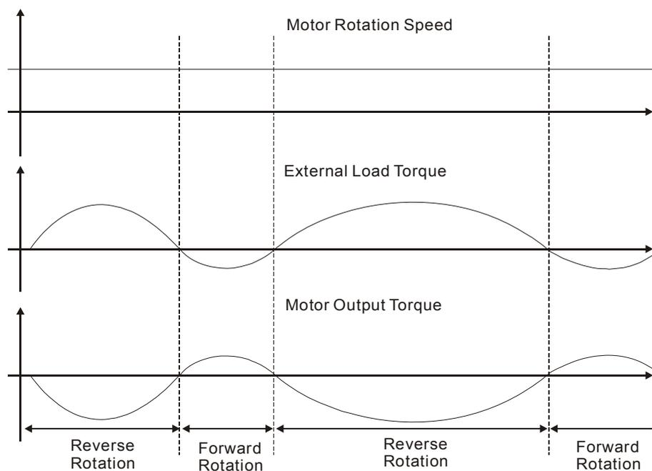
Negative torque:  $T_L \times \omega_r$      $T_L$ : external load torque
