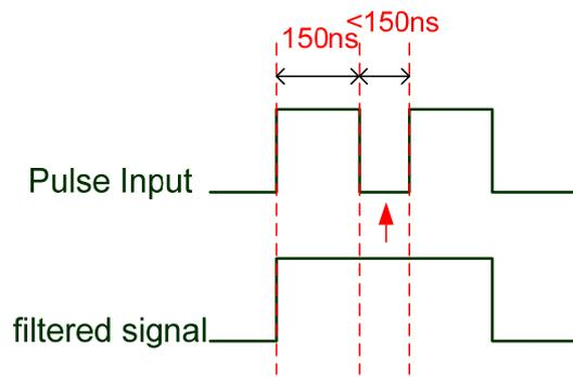
When this pulse frequency is less than 150 ns, this signal will be regarded as a high-level pulse and two input pulses will be regarded as one input pulse.
