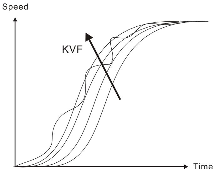
If the KVF value closes to 1, the feed forward compensation will be more complete and the dynamic following error will become smaller. However, if the KVF value is set too big, it would cause vibration.
