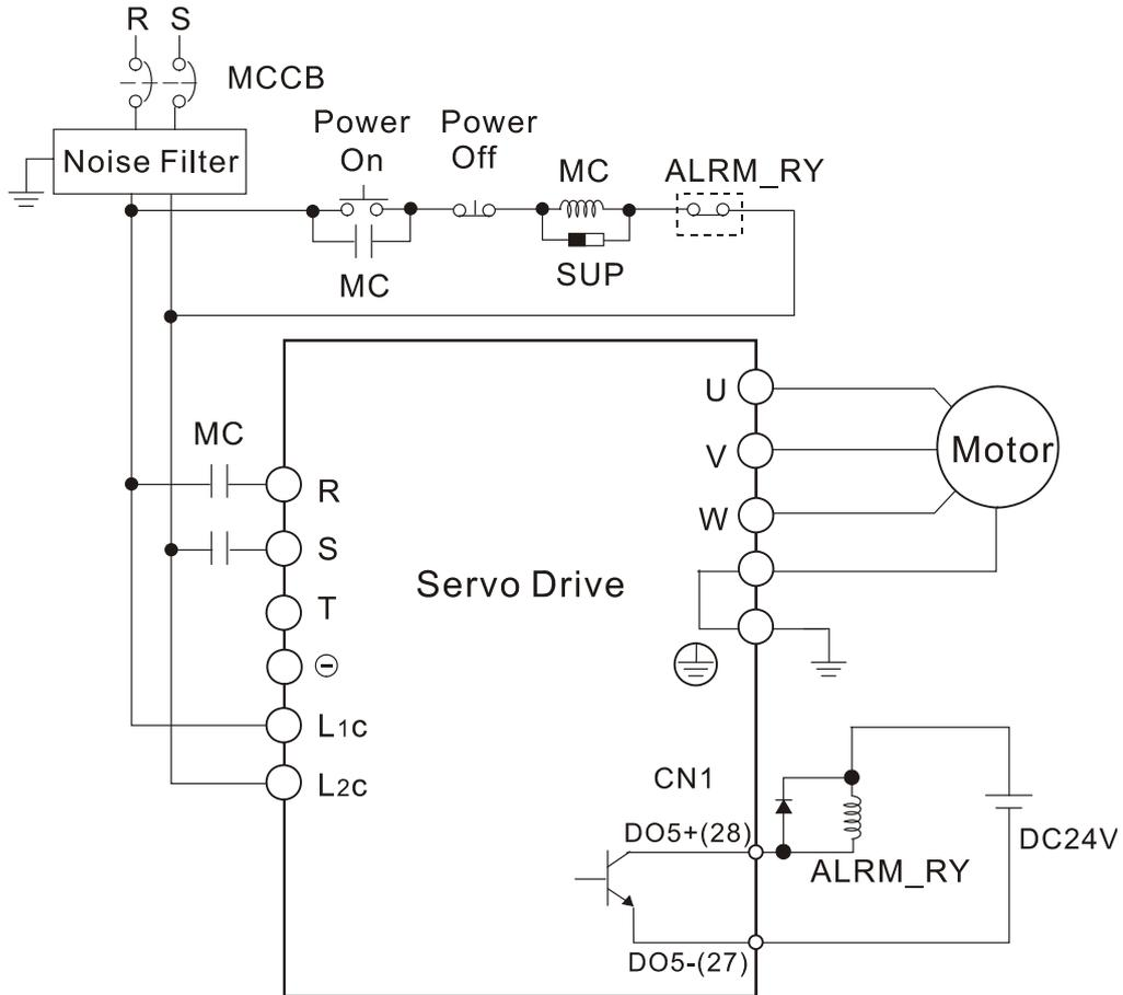
■ Wiring Method of Three-phase Power Supply (suitable for all series)
