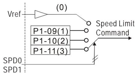
When desire to use speed limit function, users could use parameter setting or DI triggering. That is to say, set P1-02 to 0x0001 or trigger DI will do.
