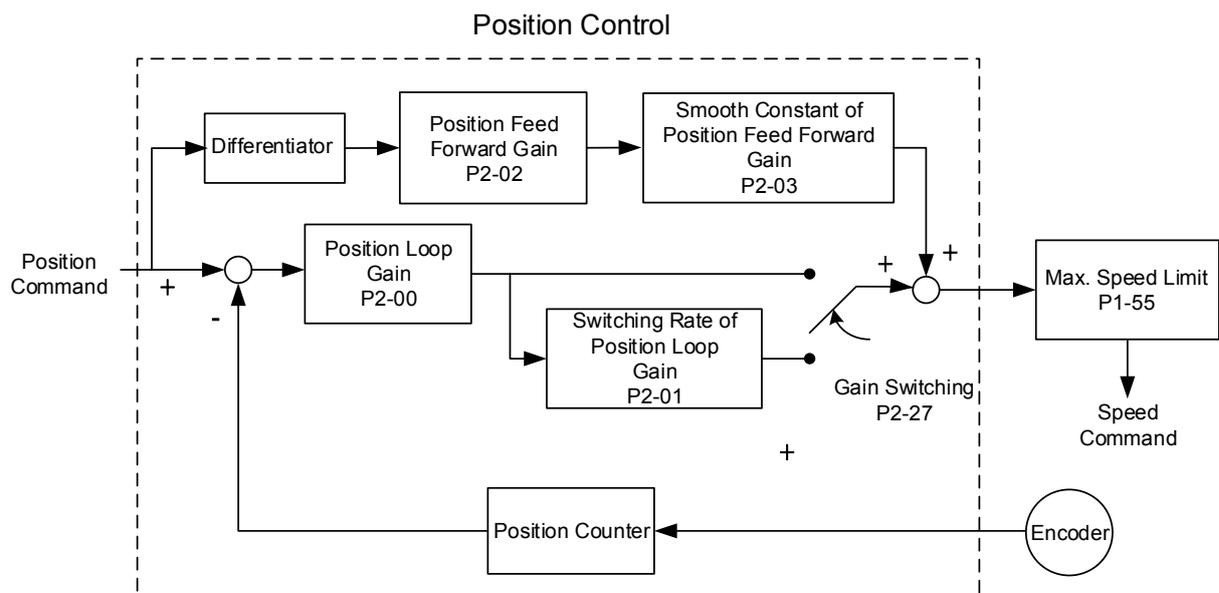
When the value of proportional gain, KPP is set too big, the response bandwidth of position loop will be increased and diminish the phase margin. And the motor rotor rotates vibrantly in forward and reverse direction at the moment. Thus, KPP has to be decreased until the rotor stops vibrating. When the external torque interrupts, the over-low KPP cannot meet the demand of position deviation. In this situation, parameter P2-02 can effectively reduce the position error.
