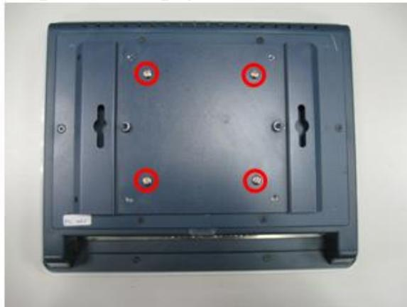
**Step 2** Assemble the VESA-ARM to the back chassis, and fix them to the GOT5152T-845 with screws (see Figure 2-18).
