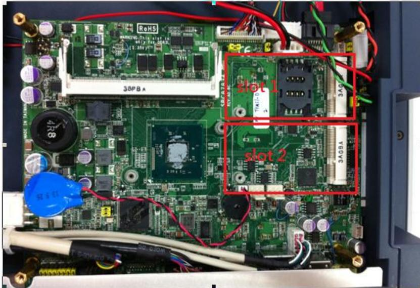
**Step 2** Insert the wireless LAN card to the slot. Screw it firmly on the slot.
