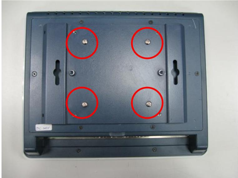
**Step 2** Assemble the VESA-ARM to the back side of the chassis, and fix the screws.
