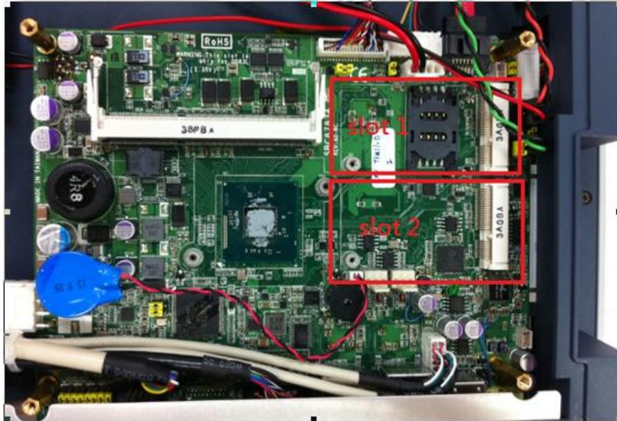
**Step 2** Insert the mSATA card to the slot 2. Screw it firmly on the slot.
