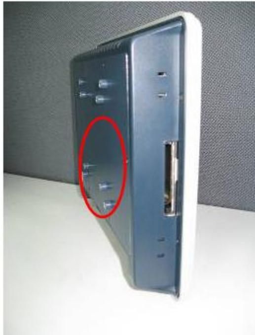
**Step 3 Locate the CFast™ socket, and insert the card into the socket.**
