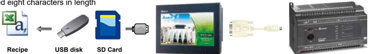
The recipe data can be saved in CSV format and easily edited on an external PC in Excel to effectively save PLC memory.
