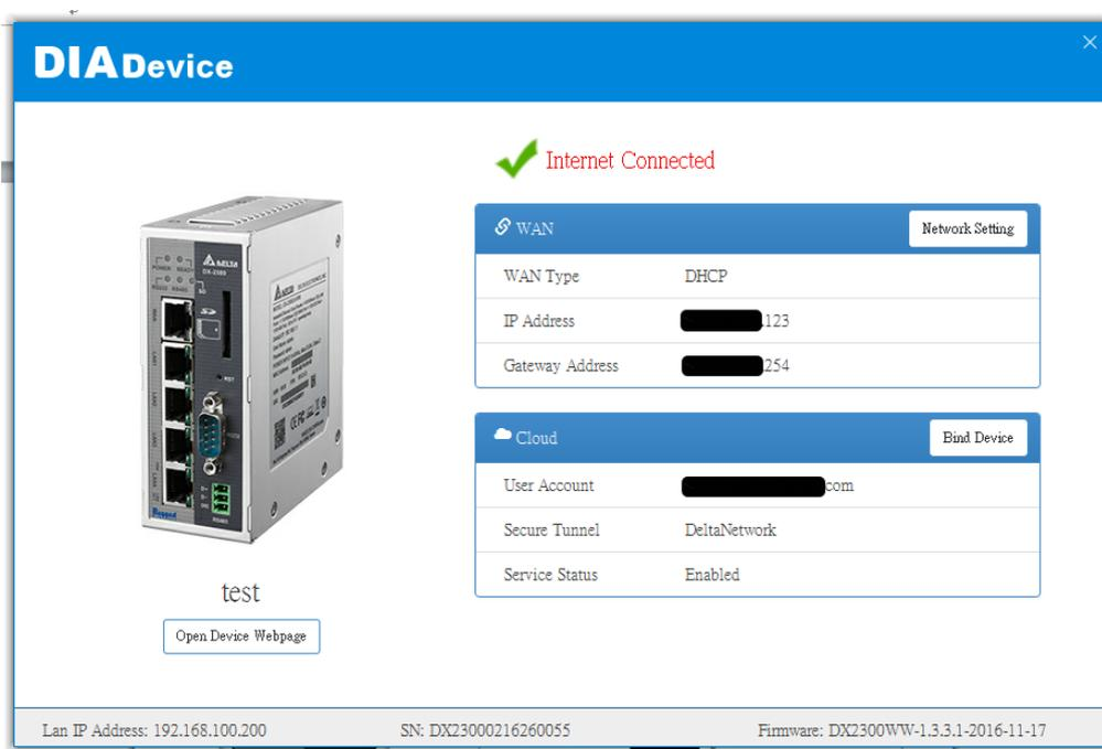
This screenshot is identical to the one above, showing the DIA Device user interface with the "WAN" and "Cloud" configuration sections. The "WAN" section shows DHCP settings for IP Address and Gateway Address. The "Cloud" section shows a User Account, Secure Tunnel (DeltaNetwork), and Service Status (Enabled). The bottom status bar displays the Lan IP Address, SN, and Firmware version.
