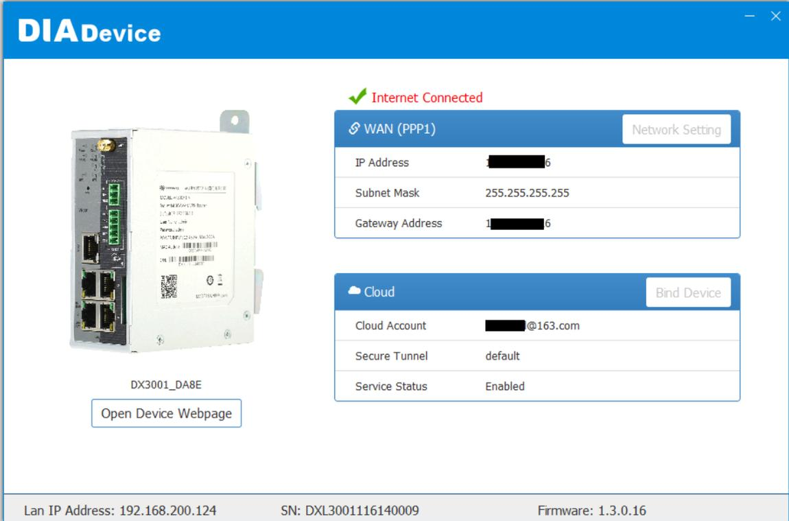
The screenshot displays the DIA Device web interface. On the left, there is an image of the DX3001\_DA8E device with a label "DX3001\_DA8E" and a button "Open Device Webpage". On the right, the interface shows a status "Internet Connected" with a green checkmark. Below this, there are two main configuration sections:
