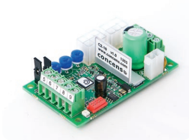
C2-10-PCB-00-0000-00 board alone, weight 36 g 73 x 42 x 26 mm (L x W x H)
