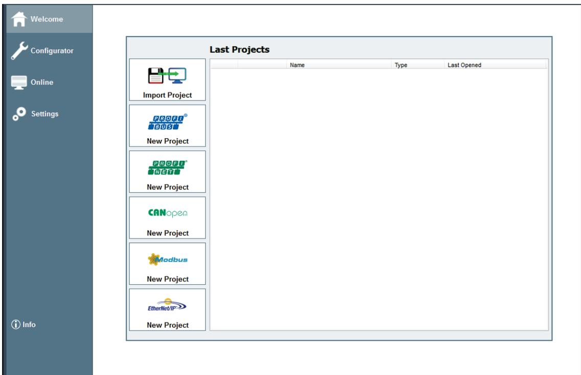
The buttons on this screen can be used to create new projects for the TB20 coupler you want or to import an existing project in the form of a file.
