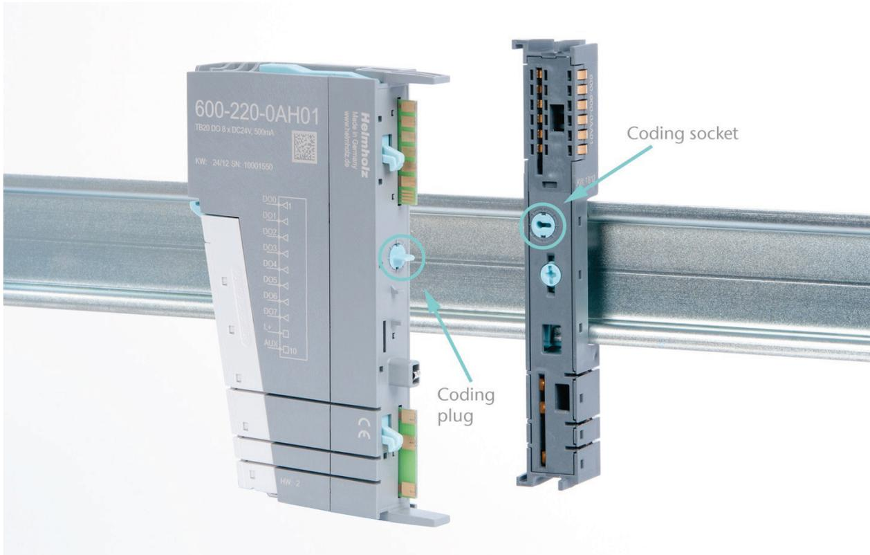
The coding plug and coding socket can each be in one of eight different positions. Each of these eight positions is factory-assigned to a specific type of module (digital in, digital out, analog in, analog out, power, etc.) from the TB20 I/O system. It is only possible to plug an electronic module into a base module if the positions of the coding plug and the positions of the coding socket match. Otherwise, the electronic module will be mechanically prevented from being plugged in.
