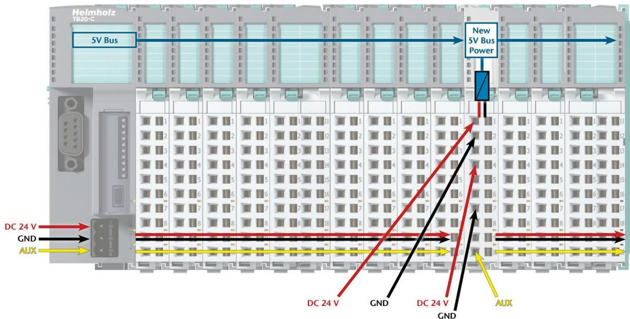
The order no. for the power module is 600-700-0AA01. Its electronic module has the same light gray color as the front connector, while its base module is light gray with a dark core.
