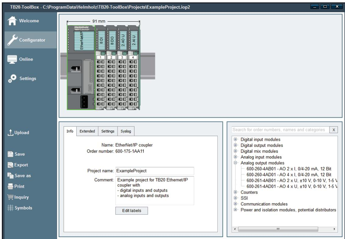
The structure view shows the selected coupler and the TB20 modules. At the bottom left, there are tabs for the module-specific information and for parameters of the selected
