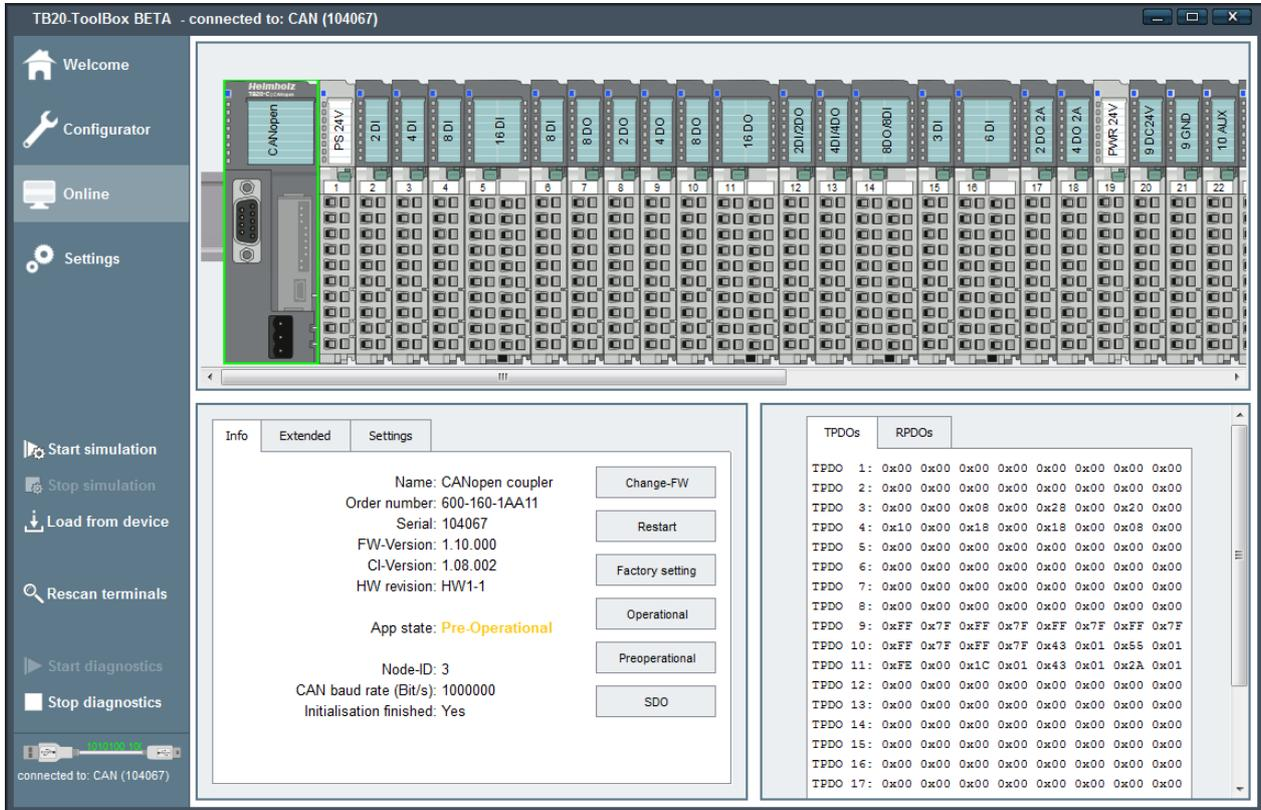
In addition to firmware updates, resetting to factory settings and the restart of the coupler the operating status can also be changed and SDOs of the coupler directly read and changed.
