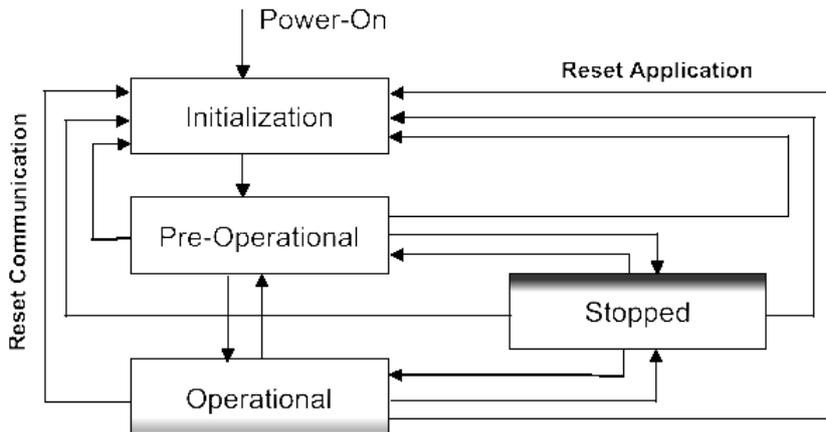
With the NMT command "Operational" [COB-ID: 000<sub>hex</sub> / data: 2 byte 01<sub>hex</sub> node ID], the coupler can be switched to **Operational** status. Once in the Operational state, the coupler's process data will be enabled (RPDO/TPDO communications will be running). However, the options available for making changes to SDOs will be limited.
