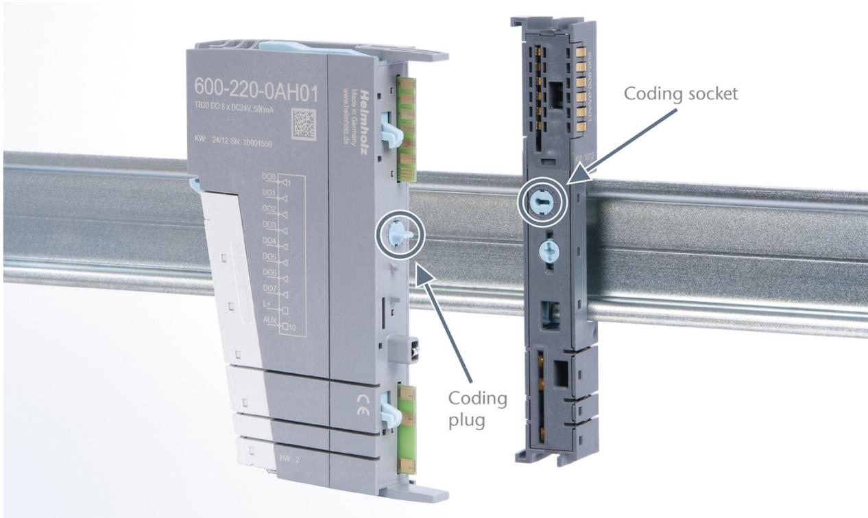
The coding plug and coding socket can each be in one of eight different positions. Each of these eight positions is factory-assigned to a specific type of module (Digital In, Digital Out, Analog In, Analog Out, Power) from the TB20 system. It will only be possible to plug an electronic module into a base module if the position of the coding plug and the position of the coding socket match. If the positions differ, the electronic module is mechanically blocked.
