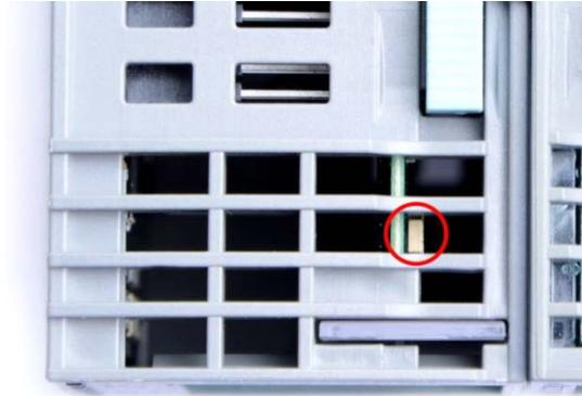
The factory settings are restored when the button is pressed while the device is powered up. As soon as the first three LEDs light up, you can let go of the button. At this point, the coupler will restart with its factory settings.
