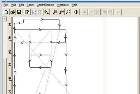
CAD2Motion is a program designed to allow users to translate CAD generated two dimensional motion paths into TrioBASIC programs.
