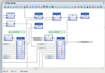
The FBD editor supports advanced graphic features such as drag and drop, object resizing and connection line routing features, so that you can rapidly and freely arrange the elements of your diagram.
