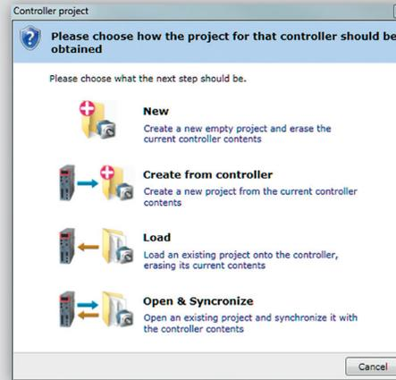
The multi-tasking capability of *Motion Coordinators* means there will be a number of different program files to make an application. In order to keep track of these multiple files and their associated data, a major component of the *Motion Perfect v4* environment is the project manager.
