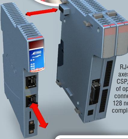
EtherCAT slave nodes are connected via the Flexslice EBUS and the EtherCAT connector (lower RJ45 socket). Up to 64 axes are supported using CSP, CSV and CST modes of operation. Total slave connections can be up to 128 nodes including I/O and complex devices.
