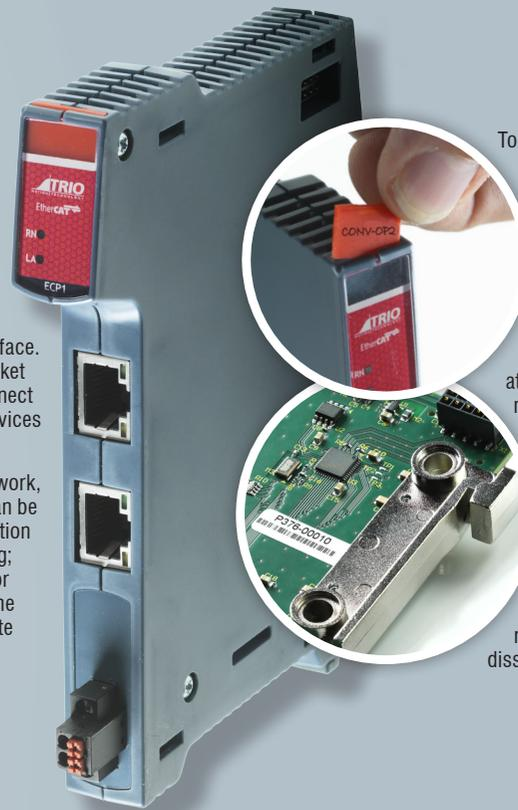
To help with identification, each Flexslice module incorporates a handy removable tab that can be written on. It simply slides in and out of a slot at the top of each module.
