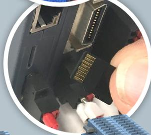
The Micro SD Card port allows the memory to be expanded to up to 32 GByte.
