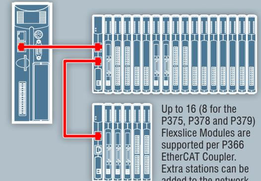
Up to 16 (8 for the P375, P378 and P379) Flexslice Modules are supported per P366 EtherCAT Coupler. Extra stations can be added to the network using the second EtherCAT port.
