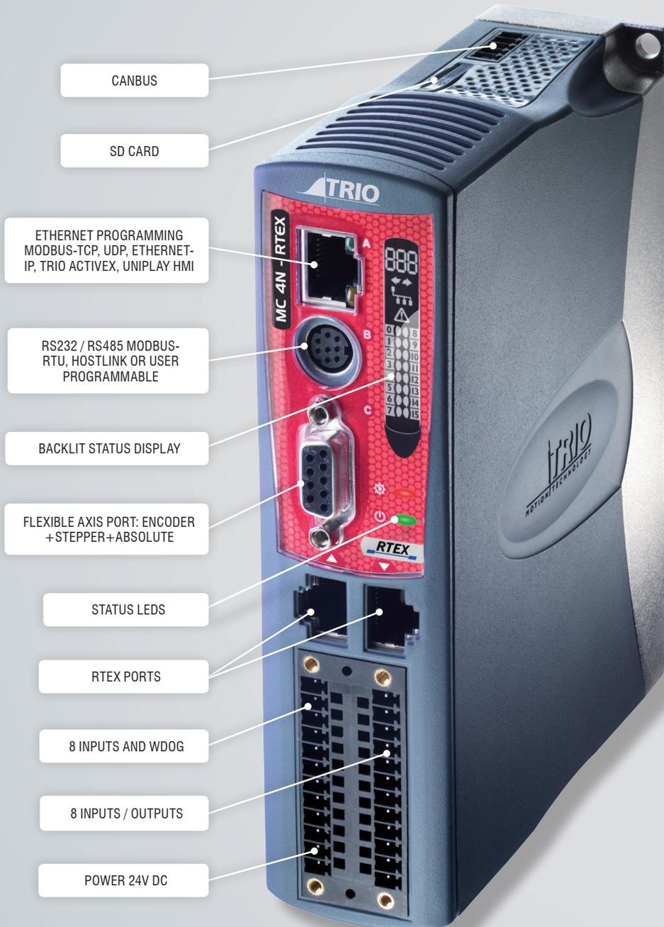
The MC4N-RTEX extends the MC4N range of *Motion Coordinators* for networked drives which started with the MC4N-ECAT. It is dedicated to running remote servo drives via Panasonic's RTEX Real Time EXpress automation bus. It is based on an up-rated version of the 532MHz ARM processor with VFP3.
