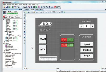
Trio's unique UNIPLAY HMI system keeps all the application programming in one place. No need for a separate HMI programming tool. *Motion Perfect v4* comes with a built in visual editor for the Trio UNIPLAY HMIs.
