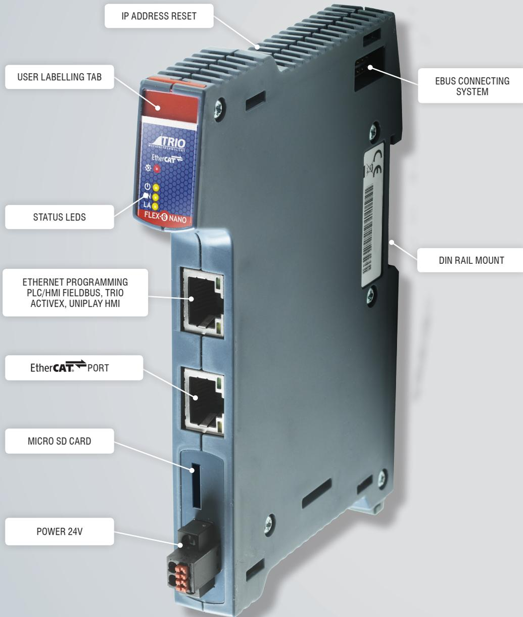
The Flex-6 Nano is a compact, integrated EtherCAT solution offering up to 64 Axes of motion. The on-board memory can be boosted to 32 GByte with the addition of a micro SD card.
