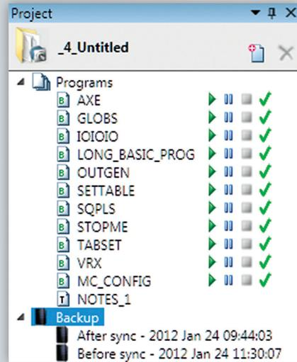
One of the keys to using *Motion Perfect v4* is its concept of a "Project". The project aids the application design and development process, by providing a copy of the multiple controller programs, parameters and data required for a single motion application, all stored in one folder.
