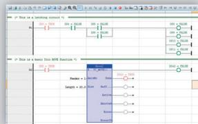
LD is probably the most widely recognised of the four supported methods because of its use in PLCs and its analogy to real world circuits. Programming in LD is best suited to applications where mostly binary variables are required and the interlocking and sequencing of digital I/O points is the primary control requirement.
