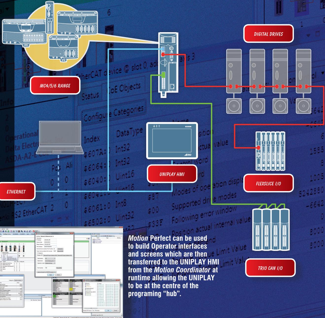
*Motion Perfect* can be used to build Operator interfaces and screens which are then transferred to the UNIPLAY HMI from the *Motion Coordinator* at runtime allowing the UNIPLAY to be at the centre of the programming "hub".
