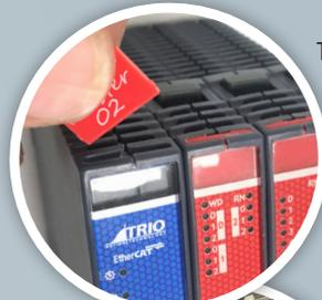
To help with identification, each Flexslice module incorporates a handy removable tab that can be written on. It simply slides in and out of a slot at the top of each module.
