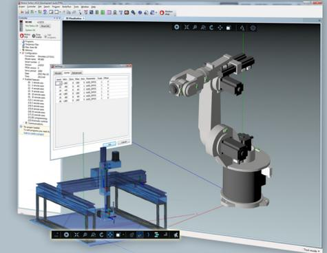
The 3D Visualization tool, available in *Motion Perfect v4*, enables simulation of Machine Motion, using an externally generated 3D model which can be synchronized with the motion program. This tool can simulate realistic movement sequences on a PC in real time.
