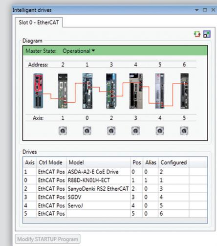
When using fieldbus axes connected to a MC4N, MC664 or MC464, *Motion Perfect v4* can access and display bus status and node specific information.
