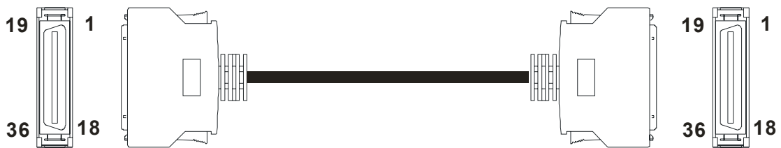
Figure 12 UC-ET010-13B ( 1M ) Female MDR36 connector ↔ Female MDR36 connector
