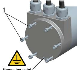
Remove the connection cap to access the terminal connectors and the dip-switches. To remove the connection cap loosen the six screws 1. Please be careful with the internal 15-pin D-SUB connector. Always replace the connection cap at the end of the operation. Take care in re-connecting the internal connector. Tighten the screws 1 using a tightening torque of approx. 2.5 Nm. Check that the encoder housing and the connection cap are at the same potential before replacing the connection cap!
