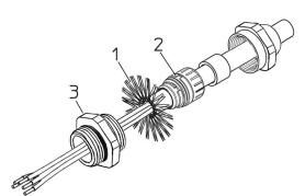
Disentangle 1 and shorten the shielding 1 and then bend it over the part 2; finally place the ring nut 3 of the connector. Be sure that the shielding 1 is in tight contact with the ring nut 3.
