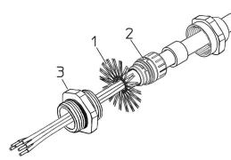
Disentangle and shorten the shielding 1 and then bend it over the part 2; finally place the ring nut 3 of the connector. Be sure that the shielding 1 is in tight contact with the ring nut 3.
