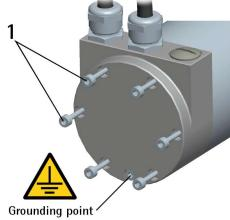
Remove the connection cap to access the terminal connectors and the dip-switches. To remove the connection cap loosen the six screws 1. Please be careful with the internal 15-pin D-SUB connector. Always replace the connection cap at the end of the operation. Take care in re-connecting the internal connector. Tighten the screws 1 using a tightening torque of approx. 2.5 Nm. Check that the encoder housing and the connection cap are at the same potential before replacing the connection cap!
