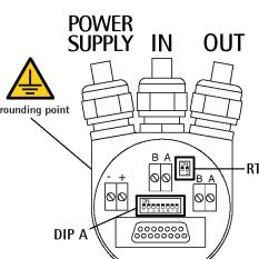
Remove the connection cap to access the terminal connectors and the dip-switches. To remove the connection cap loosen the two screws 1. Please be careful with the internal connector. Always replace the connection cap at the end of the operation. Take care in re-connecting the internal connector. Tighten the screws 1 using a tightening torque of approx. 2.5 Nm. Check that the encoder housing and the connection cap are at the same potential before replacing the connection cap!
