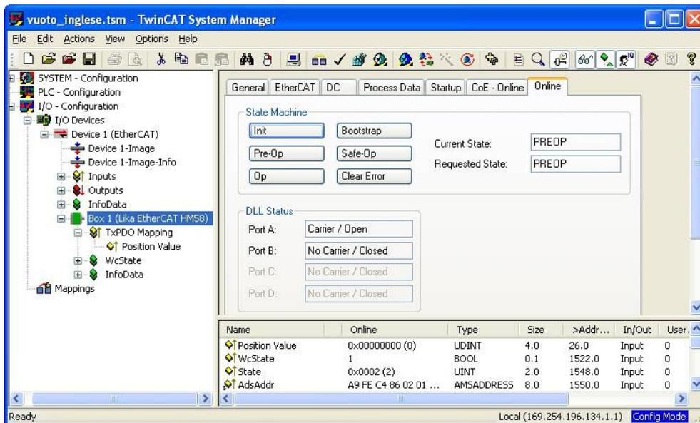
To display the encoder process data in real time, click the **Safe-OP** button if you want to display inputs only; click the **OP** button if you want to display both inputs and outputs.
