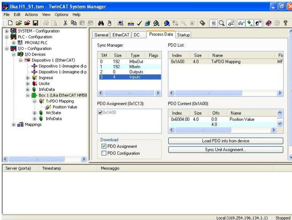
Process data objects can be displayed also by pressing the **TxPDO Mapping** item in the left pane of the **TwinCAT System Manager** main window; data is listed in the right pane.
