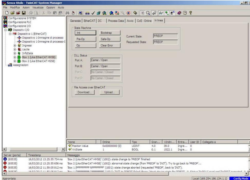
2. Press the **Bootstrap** button in the **State Machine** box; in the **BOOT** state the encoder is ready to accept the firmware upgrade download process (the **BOOT** message appears next to the **Current State** item in the same box).
