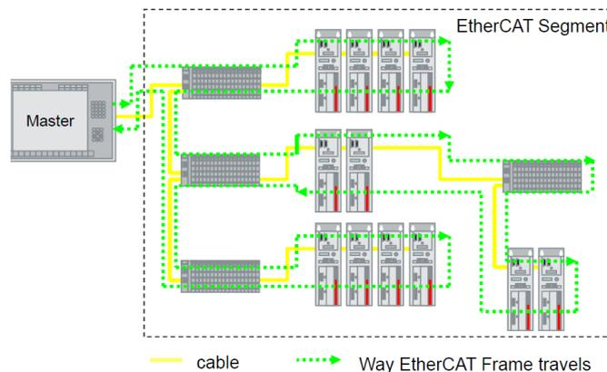
This efficient data flow is guaranteed by the 100BASE-TX full-duplex structure of EtherCAT bus which is fitted with two separated lines for transmitting and receiving data.
