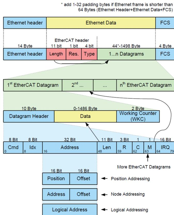
Inside the Ethernet frames data are transmitted among Master and Slaves using PDO (process data objects) protocol. Each PDO message has inside one or more addresses for issuing data to Slaves; data + address/es (and additional elements such as a validation checksum) joined together forms an EtherCAT telegram (Datagram).
