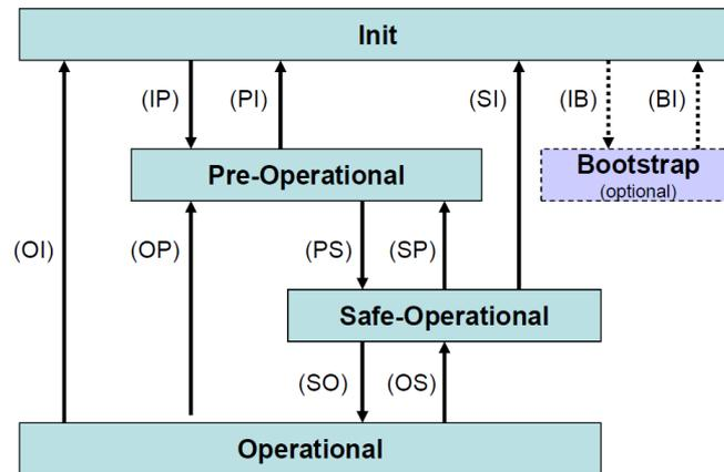
EtherCAT Slave is a state machine; communication and operating characteristics depend on the current state of the device:
