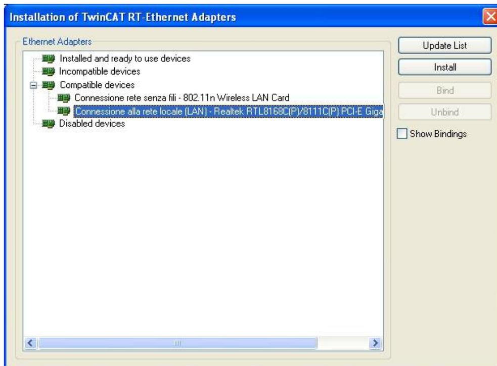
The **Installation of TwinCAT RT – Ethernet Adapter** window will appear. Now select **Compatible Devices** item and choose the network card you want to install; finally press the **Install** button to confirm your choice.
