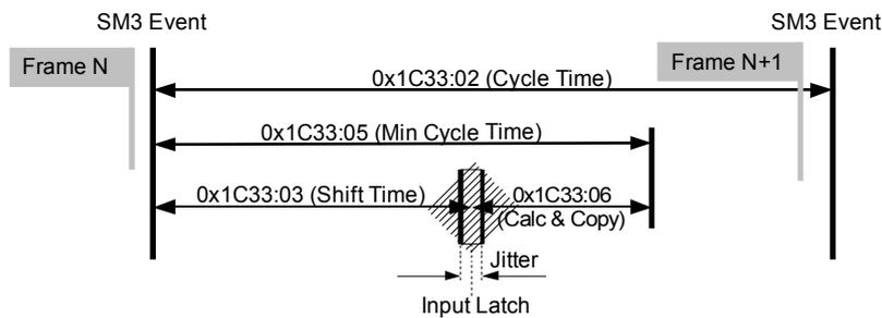
New data will be read by the Master at next cycle (following SM3 event), so if cycle time is too long, data could be relatively old for a real-time system. The main advantage is that data is updated exactly when Master is reading (synchronous mode).
