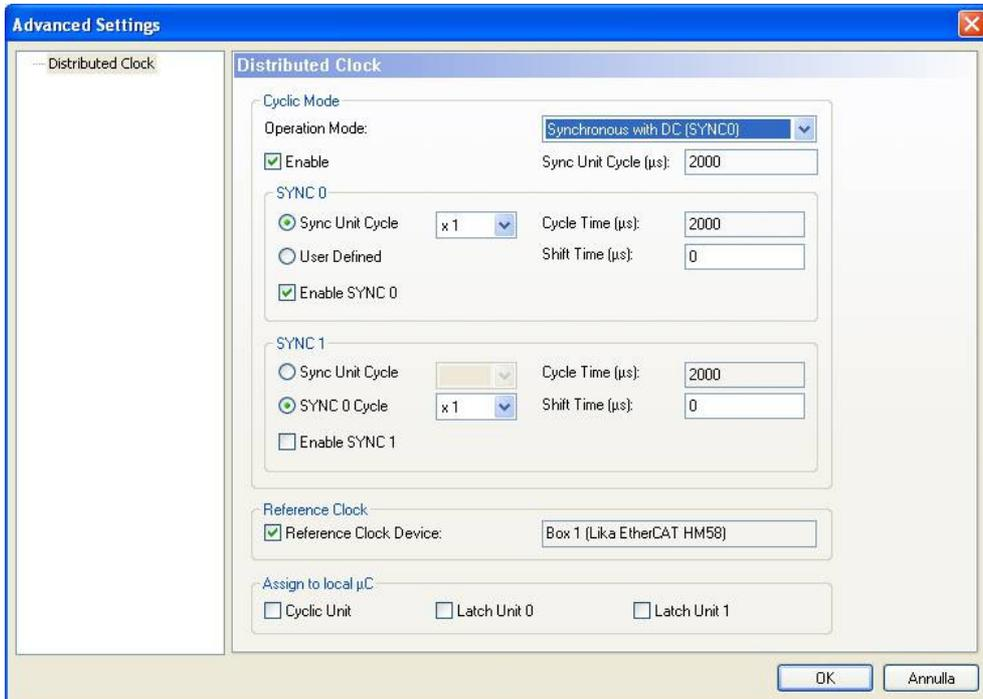
The **Advanced Settings** window will appear. In the section tabbed **SYNC 0** set the cycle time next to the **Sync Unit Cycle** box; sync time is calculated as multiple (or sub-multiple) of the value set in the **Sync Unit Cycle (µs)** item right above.
