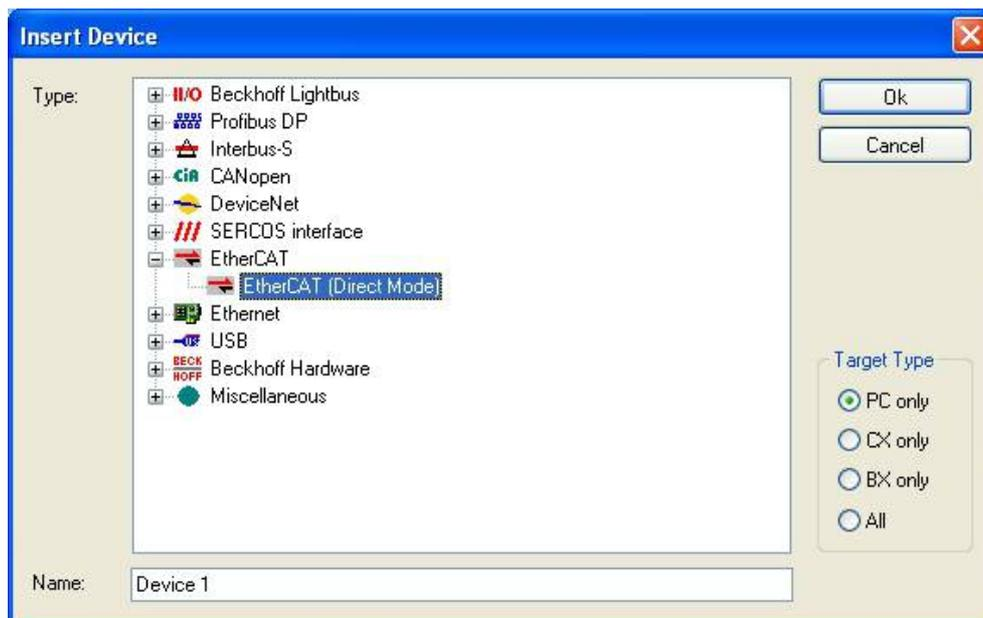
If a network card has been already installed properly, the following window will appear showing the list of the installed devices.
