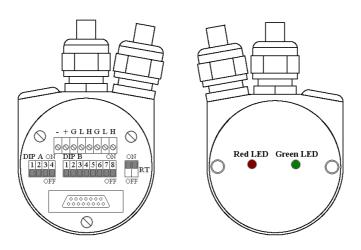
The connection cap is fitted with two PG9 cable glands for bus-IN, bus-OUT and supply voltage connections. The bus cables can be connected directly to the terminal connectors in front of each cable gland. It is recommended to use CANbus certificated cables. Core diameter should not exceed  $\emptyset$  1,5 mm (0.06 inches).
