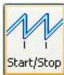
**Programming mode: Start / Stop (cyclic ramp):** TEACH IN, it allows to programme the encoder by considering directly the physical travel of the application you need to measure and control; the travel is defined in a ramp which is then repeated cyclically: as soon as the the final position of the travel is reached, then the minimum signal level of the selected range is output to start a new ramp, see on page 47.
