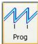
**Programming mode: Prog (cyclic ramp):** it allows to programme the encoder provided that you know exactly the number of encoder information (counts) for the physical travel of the application you need to measure and control; the travel is defined in a ramp which is then repeated cyclically: as soon as the the final position of the travel is reached, then the minimum signal level of the selected range is output to start a new ramp, see on page 52.
