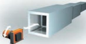
In combination with telescope-like systems, wire-actuated encoders can be ideally integrated and are also protected from environmental impact.
