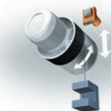
Direct position feedback after winch adjustment. The wire-actuated encoder can be positioned outside danger or humidity areas by means of wire extension.
