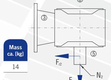
The mass of the gearbox may deviate depending on the flange size, the type and the gear ratio.
