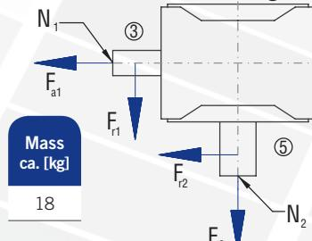
The mass of the gearbox may deviate depending on the gear ratio and the type.
