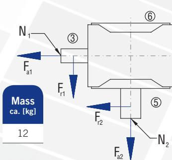
The mass of the gearbox may deviate depending on the gear ratio and the type.
