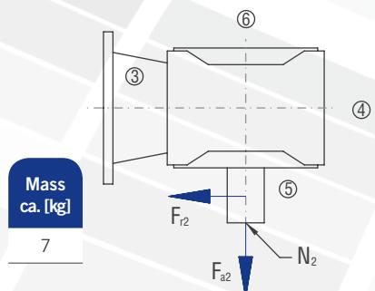
The mass of the gearbox may deviate depending on the flange size, the type and the gear ratio.
