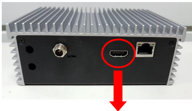
HDMI connector (PICO512-CN15) on rear side
