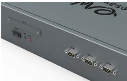
Side A - Detail of CFast slot , serial ports and main power push button switch.
