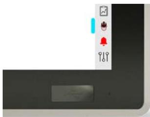
Detail of true-flat touch screen along with twisted aluminum bezel and ATEX IP66 frontal USB port.
