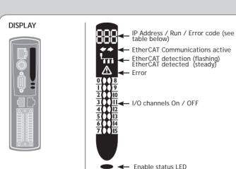
The IP address and subnet mask of the MC4N is shown on the LCD display for a few seconds after power-up. The factory default IP address is 192.168.0.250. This can be changed using the IP\_ADDRESS command via the *Motion* Perfect v3 software tool.
