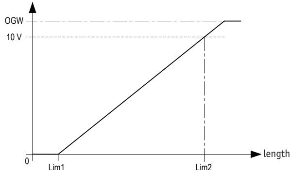
Fig. 5: signal sequence voltage output (e.g. 0-10 V)
