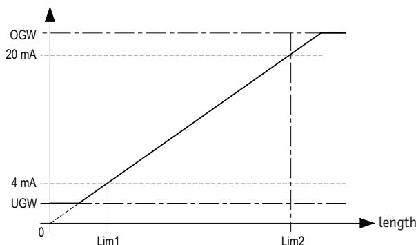
Fig. 6: signal sequence current output (e.g. 4-20 mA)
